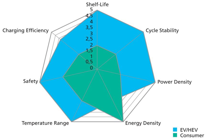
compares the main features of common consumer cells to new cells containing Lithiumtitanate as anode material.
