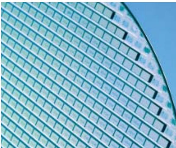
Silicon Wafer with encapsulated micro mechanical gyroscopes.
