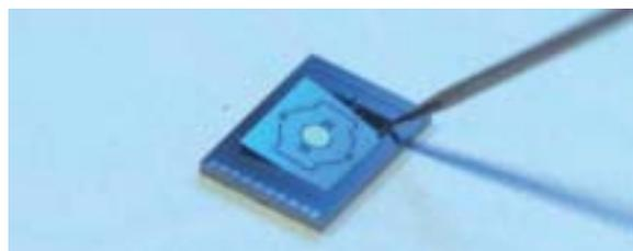
Figure 2: A new mirror design enables permanent static preinclination of the 2D-scanner for spatial separation of reflex and projected image.
