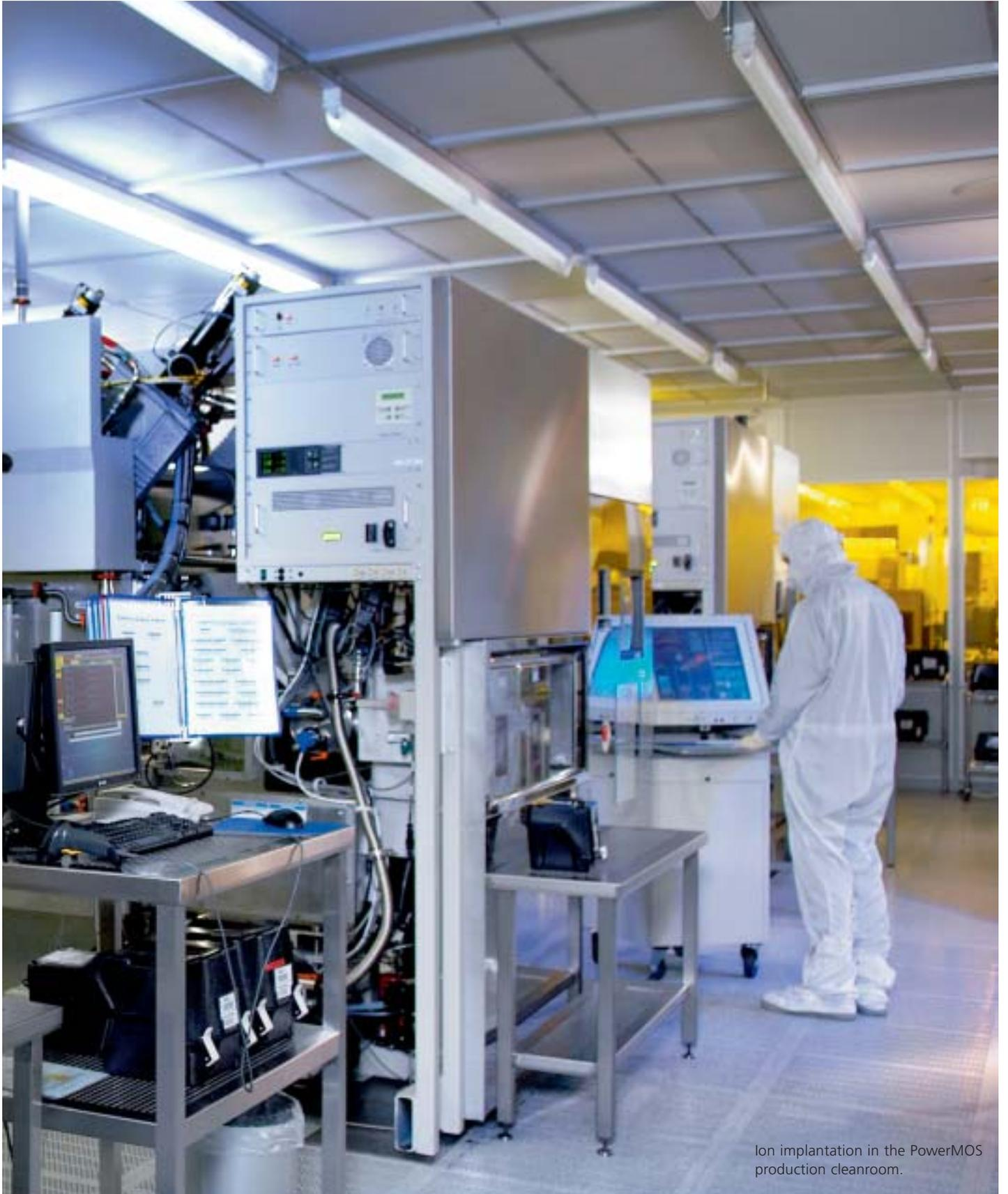
Ion implantation in the PowerMOS production cleanroom.
