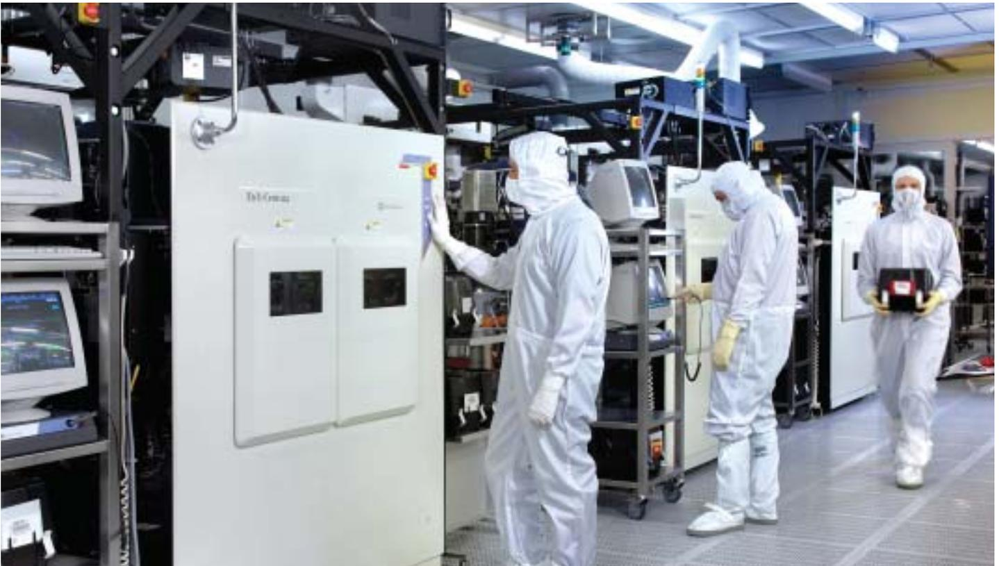
Reactive Ion Etching (RIE) tools in the PowerMOS production cleanroom.
