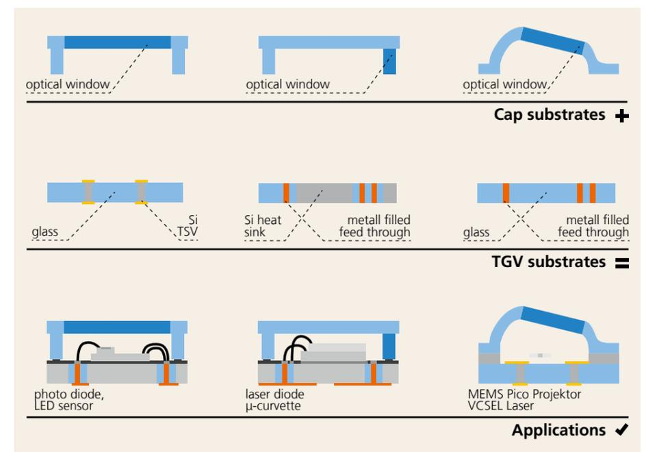
Schematic of different optical housing constructions supported by the modular packaging system
