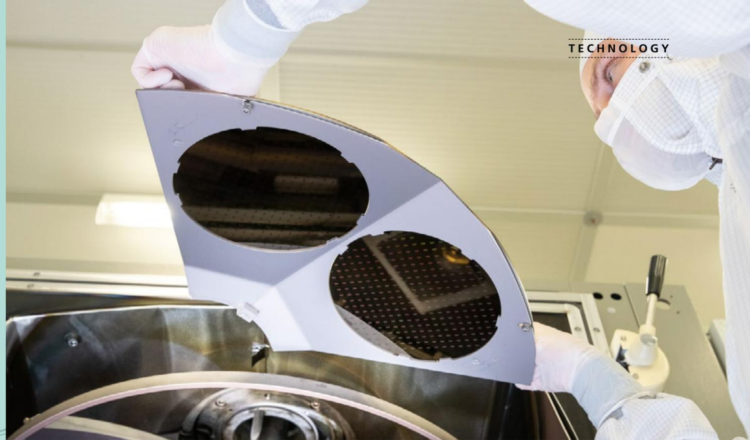
Operator loading wafers into the evaporation chamber
