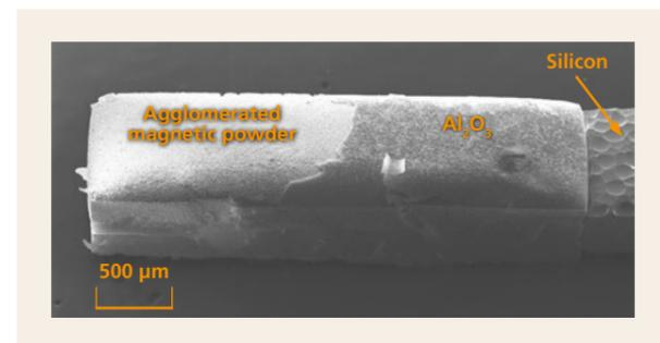
Figure 2: SEM image of the core P04, after partly removal of the surrounding silicon by etching in  $\text{XeF}_2$  gas phase
