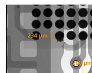
Figure 4: Molten solder ball
