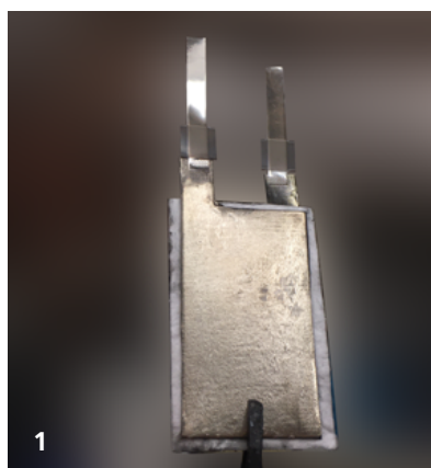
1 Demonstration of the world's first calcium ion cell in pouch technology
