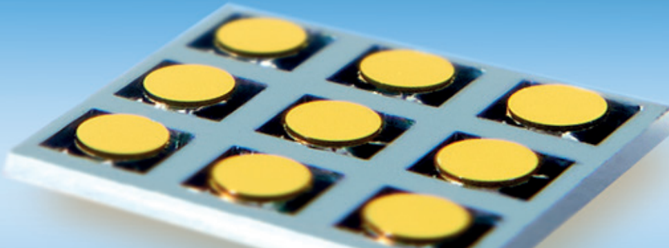
1 Array of nine piezoelectric, quasi-static MEMS mirrors with gold reflector
