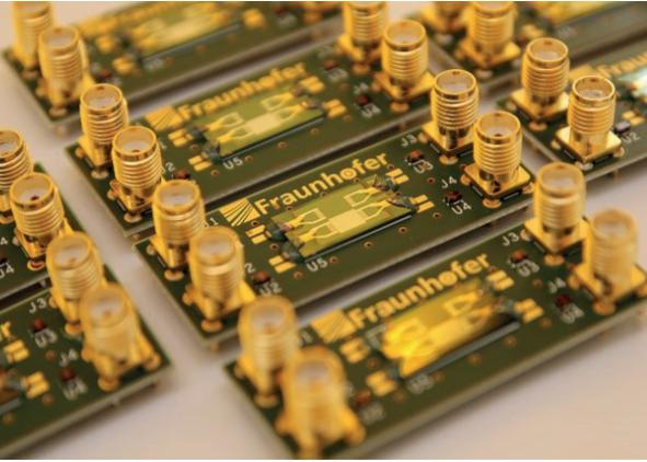
Test PCB with SAW magnetic field sensor
