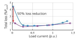
Power loss reduction with GaN based auxillary circuit
