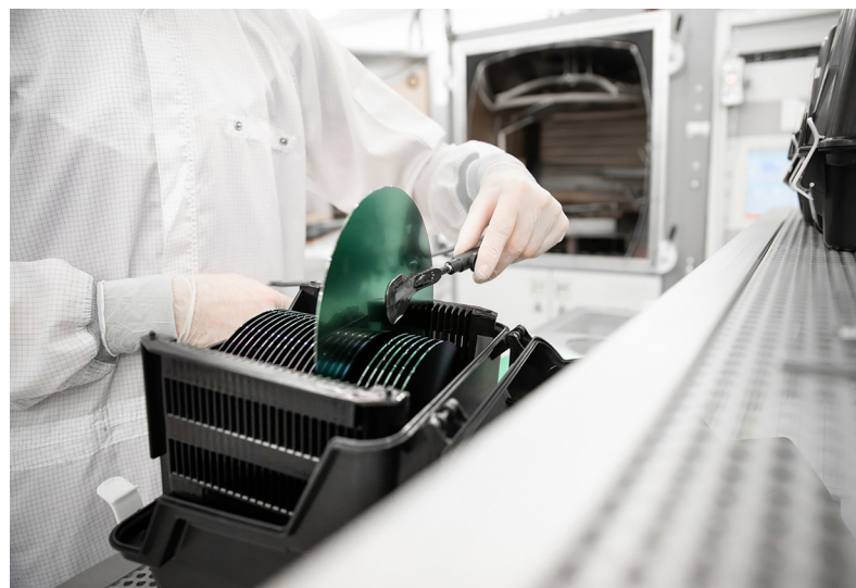
Handling of 8-inch wafer in clean room
