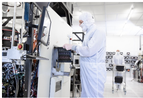
©Fraunhofer ISIT – Post-CMOS clean room at Fraunhofer ISIT for GaN and MEMS device development.
