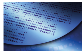
200 mm Si Wafer with integrated NdFeB micromagnets
