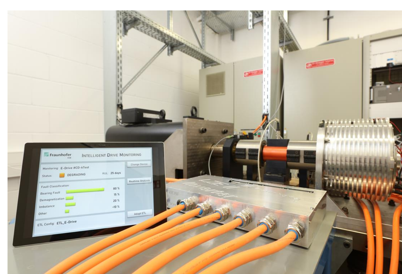
Motor-test bench (© Kurt Fuchs, IISB)
