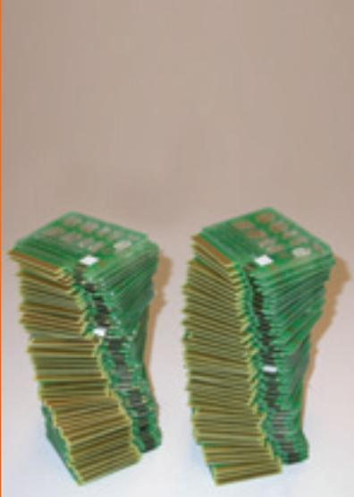
Figure 2a: ivD-cartridges equipped with microfluidics and chip
