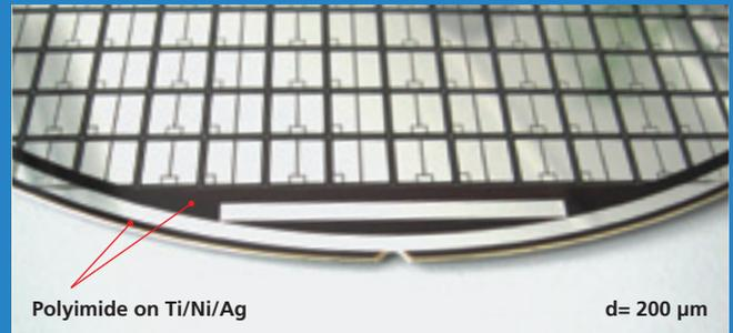
Figure 4: AlCu/Ti/Ni/Ag wafer- surface with Polyimide insulation of 20  $\mu\text{m}$  thickness
