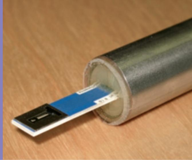
Figure 13: Sensor set up on ceramic in a steel pipe
