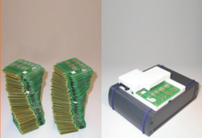
Figure 2a: ivD-cartridges equipped with microfluidics and chip
