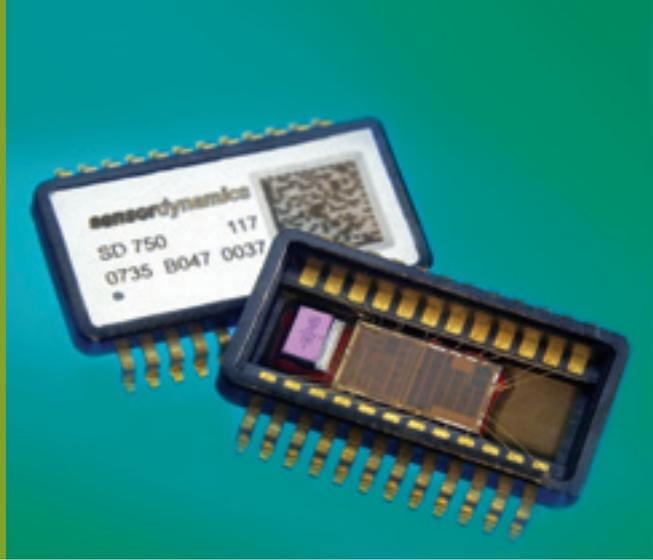
Figure 1: Gyro modul: Sensorchip and ASIC in open cavity package
