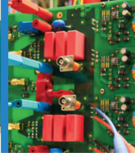
Figure 3: DC/DC-converter with > 99 % efficiency
