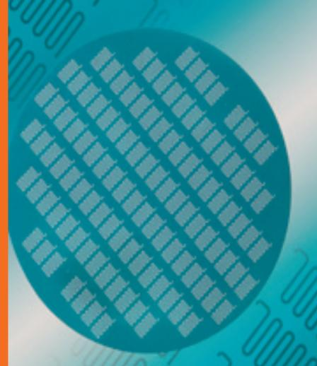
Figure 3: Silicon wafer with "on-chip" porous separation columns
