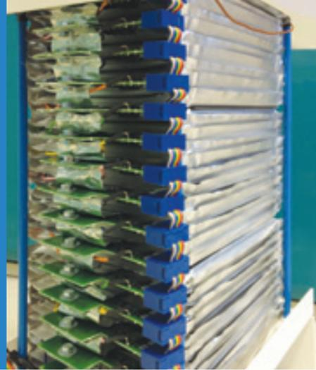
Figure 2: Battery storage system with Li-Titanate cells
