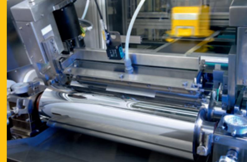
Traversing contact-free coating thickness control (yellow) at the coater in the pilot plant
