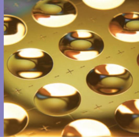
Figure 4: Detail view of gold covered reflector surfaces on 8"-glass-wafer
