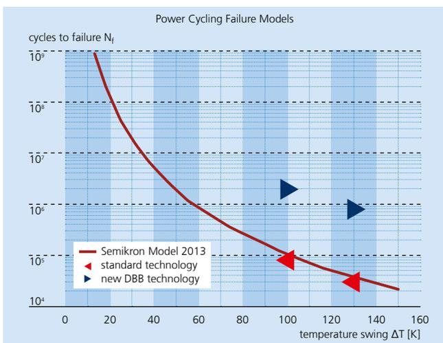
Figure 4: Comparison of reliability results by power cycle tests (blue: DBB Cu wire bonds, red: Al wire bonds)
