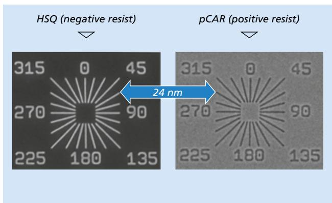
Figure 9: 24 nm lines show any angle capability (Source: IMS Nanofabrication AG)
