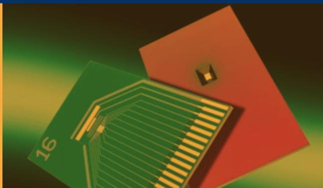
*Microfluidic chip with electrodes for electrochemical analyses*
