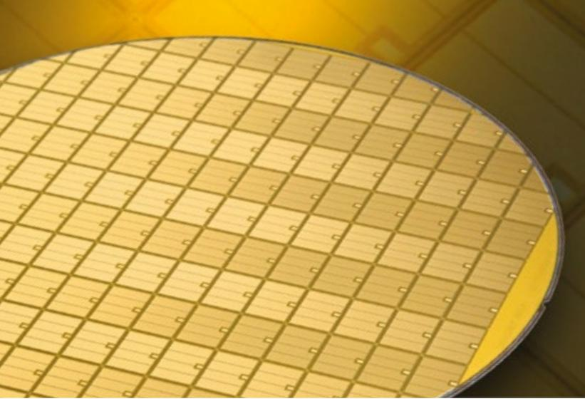
Figure 2: Top view of a 1200 V/200 A IGBT wafer with Ni-Au metallization for DBB assembly technique
