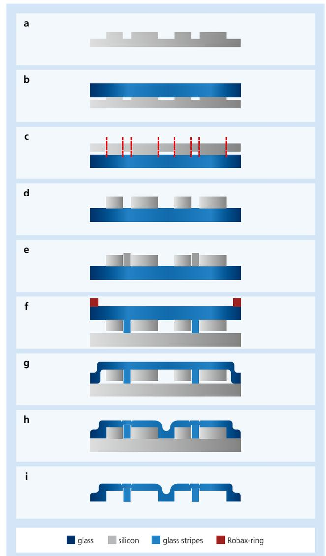
Figure 2: Schematic of the process flow for the glass wafer with vertical windows
