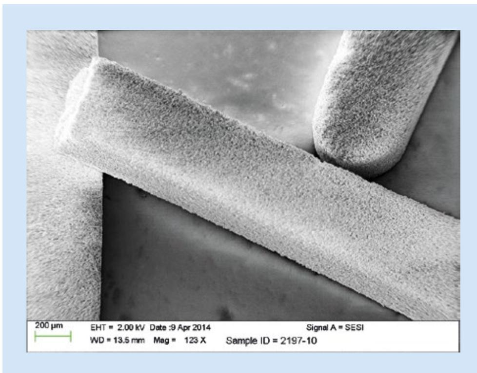
Figure 2: Electron microscopy of a processed porous column (removed from the Silicon carrier)
