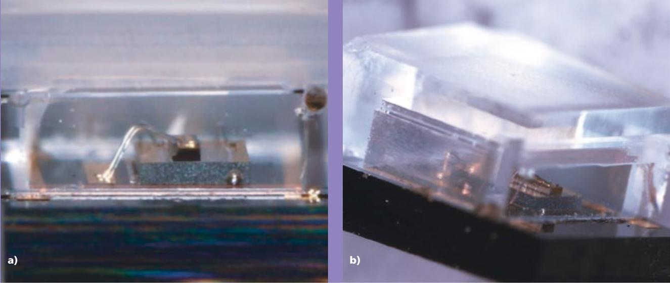
Figure 5: Front view (a) on a mounted laser diode on a submount through the vertical emission window; b: side view
