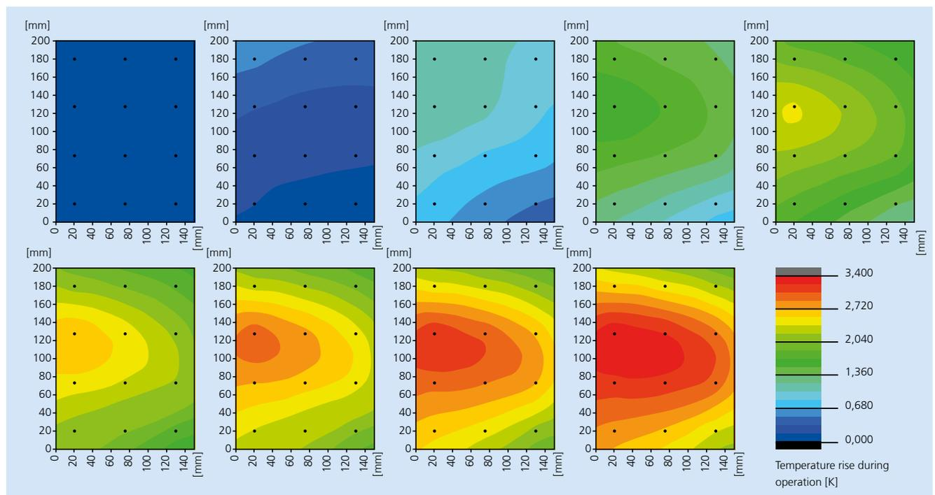
Figure 3: Evolution of the temperature distribution in a rectangular pouch-cell (151 x 200 mm<sup>2</sup>) during the 2C charge operation, measured with temperature sensors inside the cell. The different graphs show temperatures at SOC = 0%, 15%, 30%, 45%, 60%, 70%, 80%, 90%, 100%
