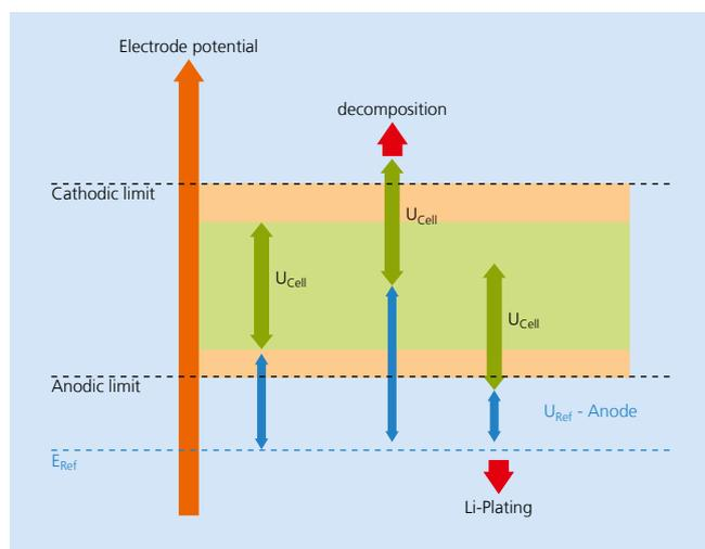
*Figure 1: Schematic view of the potential ranges in an electrochemical cell. When the potential of both electrodes is shifted, the potential limits could be exceeded although the cell voltage is inconspicuous*
