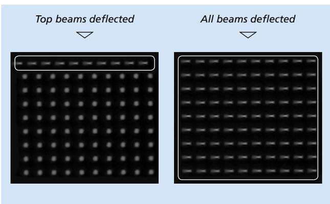
Figure 8: Deflected and undeflected beam images from a scintillator detection plate. (Source: IMS Nanofabrication AG)
