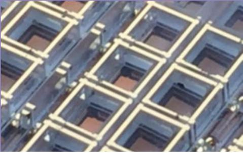
*Figure 3: Detail view of a separated 8" glass cap wafer with vertical emission windows, multilayer anti-reflective coating and deposited plating base*
