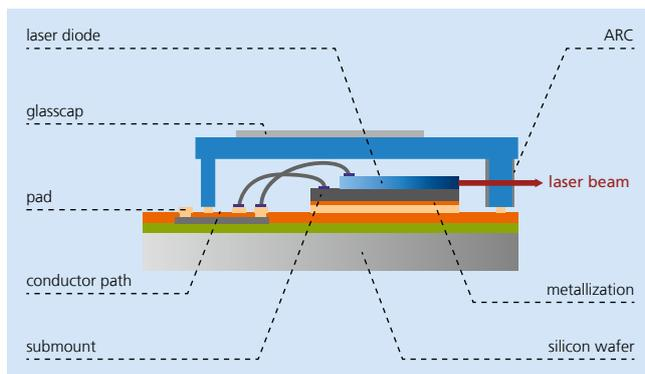
Figure 1: Schematic construction of a miniaturized laser module with lateral emission window
