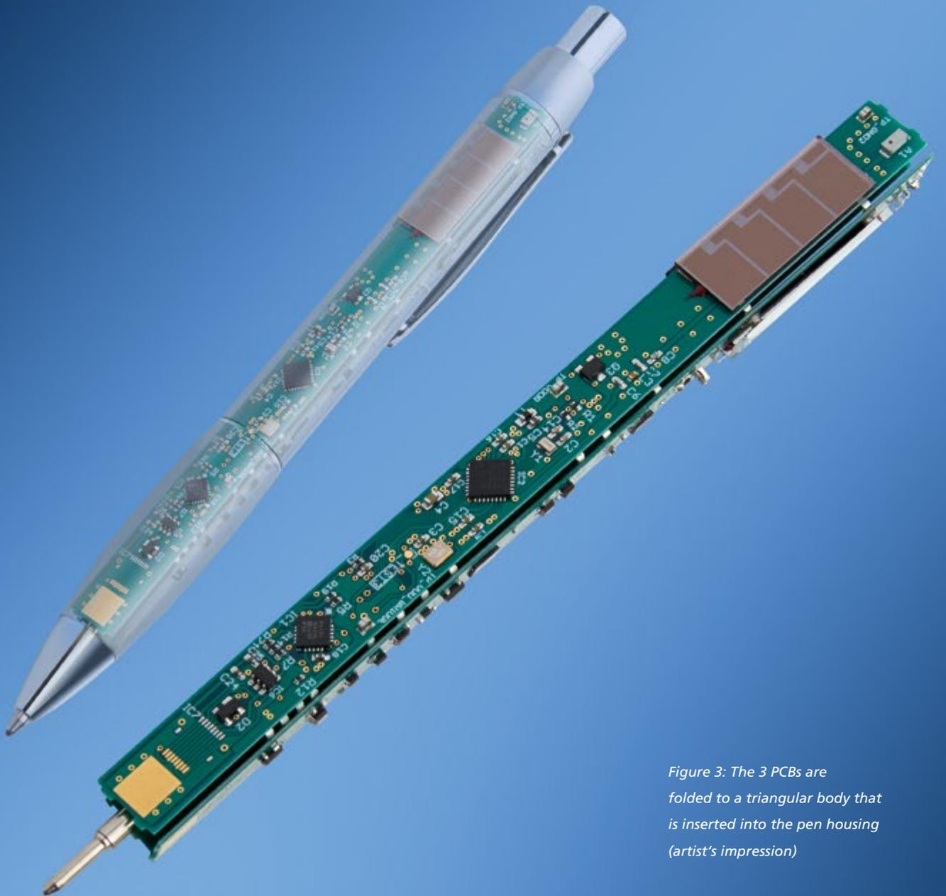
Figure 3: The 3 PCBs are folded to a triangular body that is inserted into the pen housing (artist's impression)
