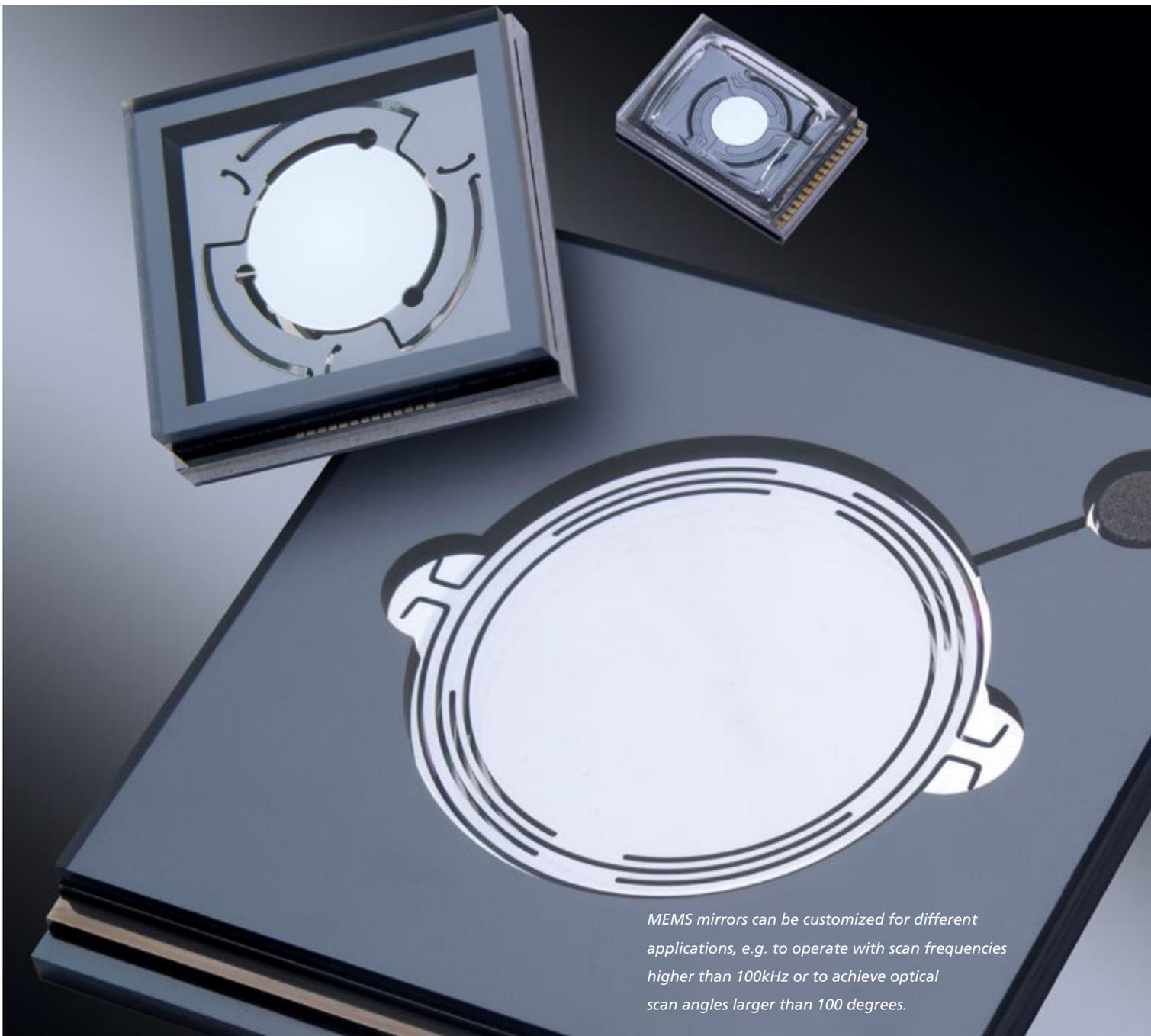
*MEMS mirrors can be customized for different applications, e.g. to operate with scan frequencies higher than 100kHz or to achieve optical scan angles larger than 100 degrees.*
