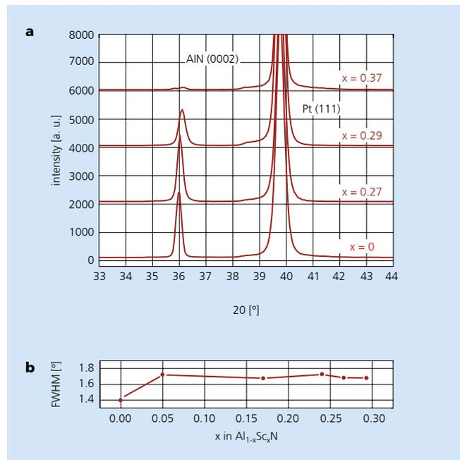
Figure 3: (a) X-ray diffraction patterns for samples with varying Sc content from  $x=0$  to  $x=0.37$  and (b) corresponding rocking curve
