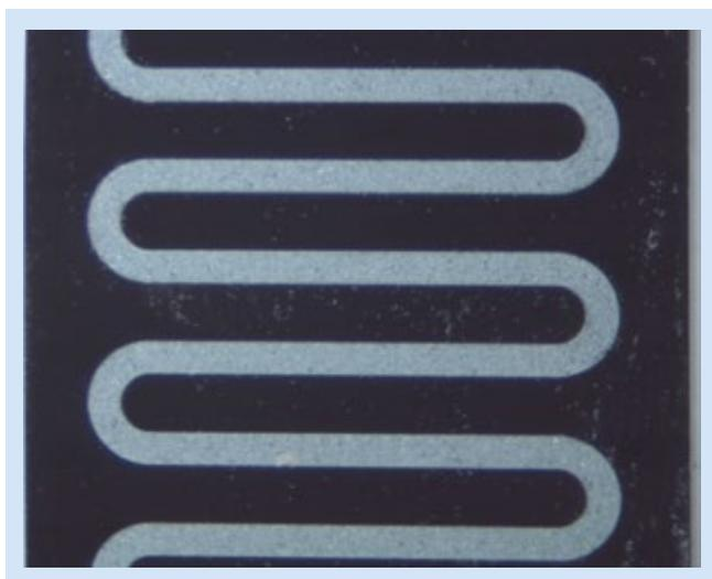
Figure 4: Separator column formed by sintered porous Silicon ceramic
