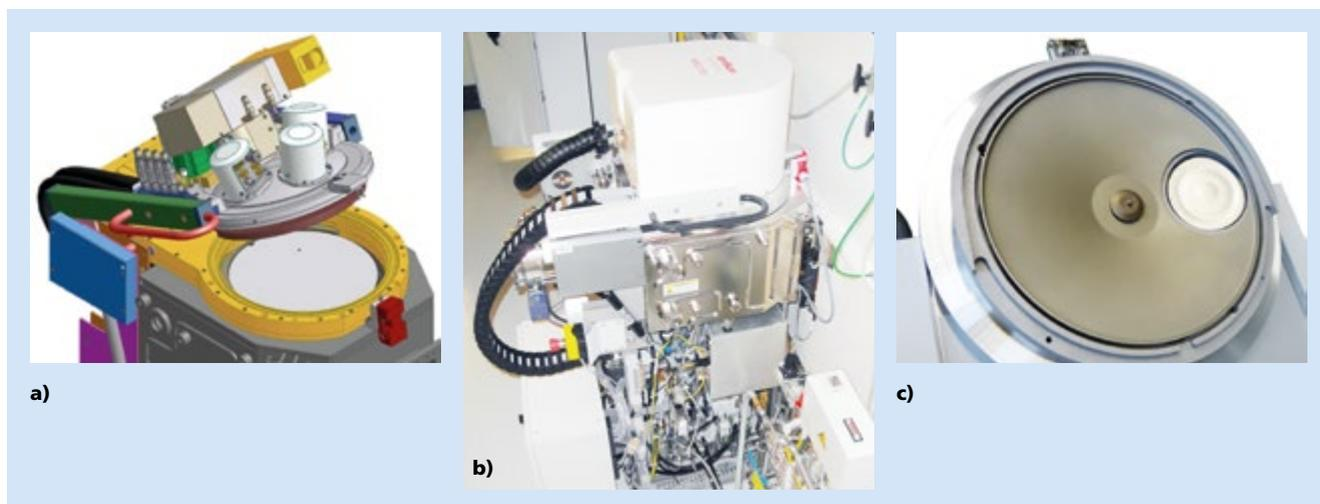
Figure 1: (a) sketch of the substrate electrode arrangement and different sources on top; (b) image of the Evatec MSQ 200 single module; (c) view on the upper chamber part with target shutter for single target deposition
