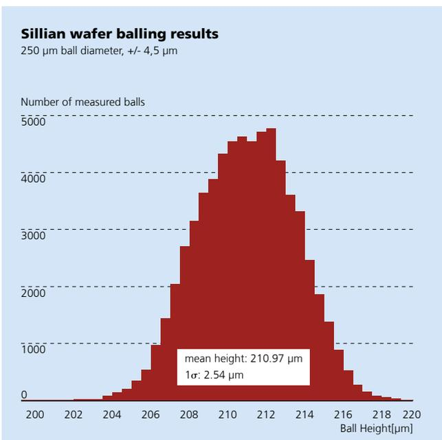
Figure 3. Ball size distribution after reflow using 250  $\mu\text{m}$  balls with 4,5  $\mu\text{m}$  tolerance (3 sigma) on 146  $\mu\text{m}$  UBM pads
