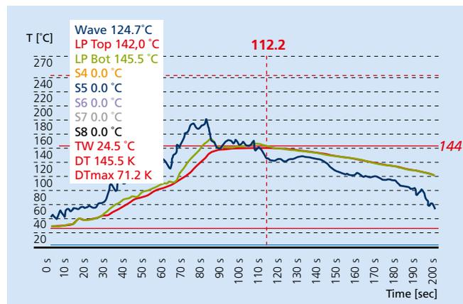
Figure 3: Incomplete wave soldering profile; max. temperature: PCB Bottom 153°C, PCB Top 142°C
