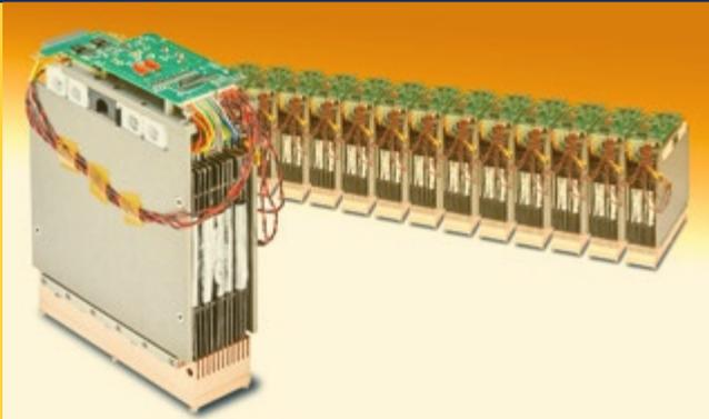
*Lithium booster battery module with 12 high performance cells and integrated electronics; background: complete battery*
