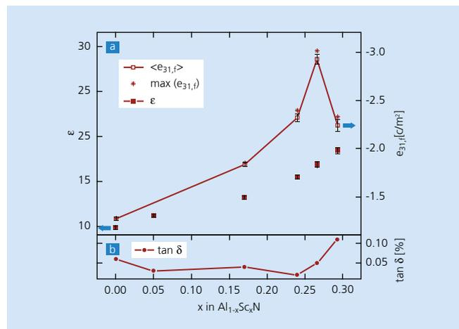
Figure 4: Mean and maximal transversal clamped piezoelectric coefficient  $e_{31,f}$ , dielectric constant  $\epsilon$  and (b) dielectric loss tangent of  $Al_{1-x}Sc_xN$  as a function of Sc content
