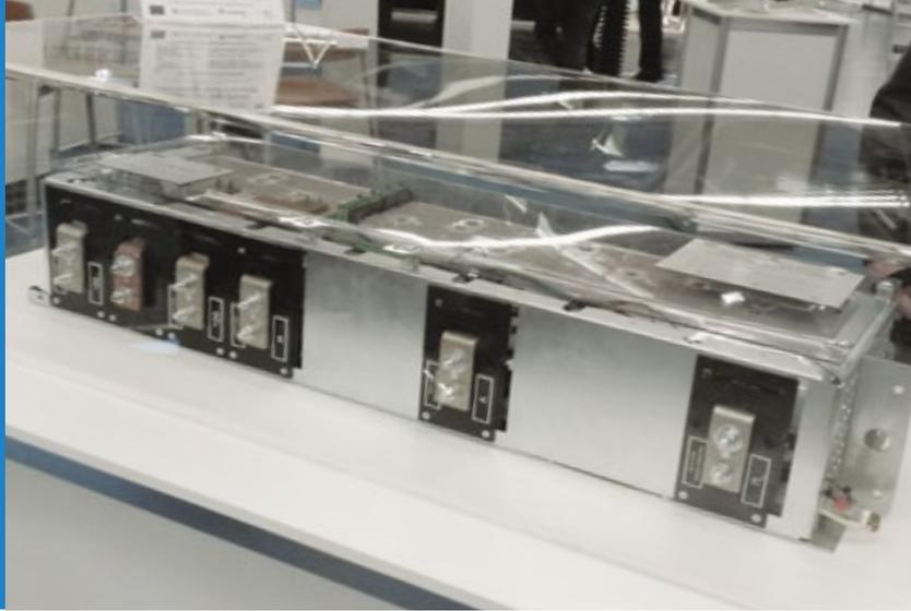
Figure 5: 3-level NPC power stack for 1MW developed by the Innovationcluster Power Electronics for Renewable Energy (Exhibition PCIM 2015)
