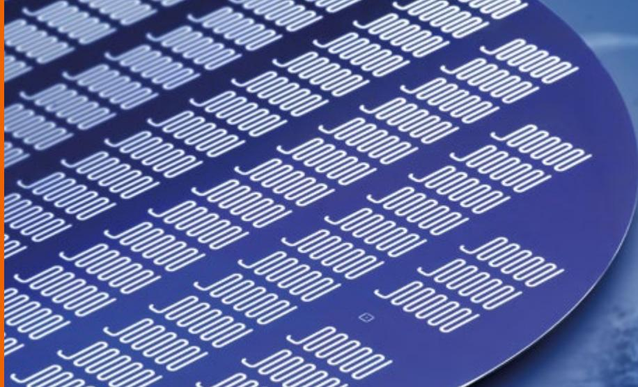
Figure 3: Silicon wafer with "on-chip" porous SiO<sub>2</sub> separation columns
