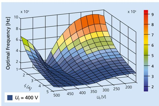
Figure 2: Optimal switching frequency
