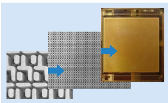
*Figure 6: Detail and overview of electrode arrangement and top view of electroplated electrodes close to apertures*
