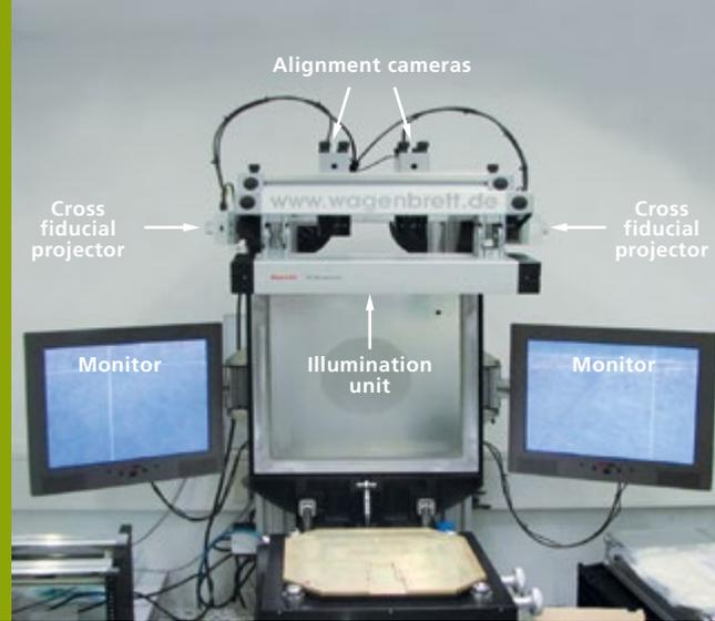
Figure 1: Wafer solder balling machine Wagenbrett WB300
