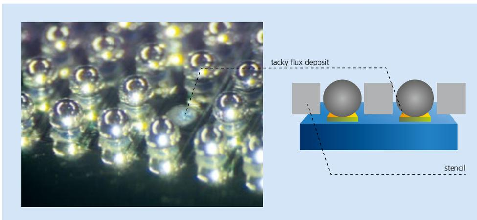
Figure 2: Solder spheres are placed on a wafer via a balling stencil and held in place by tacky flux deposits
