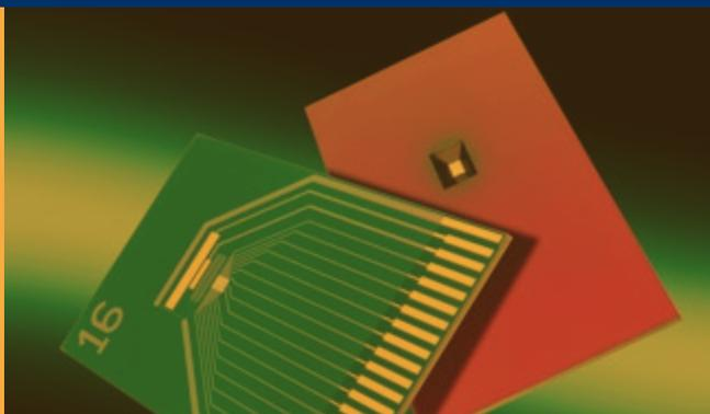
*Microfluidic chip with electrodes for electrochemical analyses*
