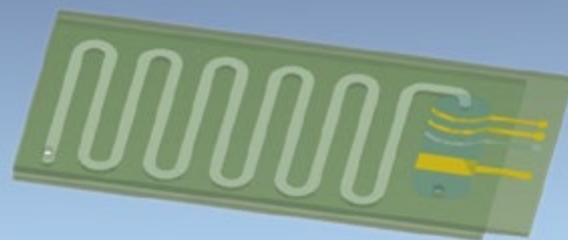
Figure 1: Construction scheme of the chromatography chip
