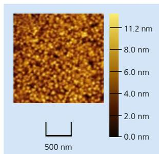
Figure 2: AFM scanned topography of a  $Al_{0.73}Sc_{0.27}N$  sample
