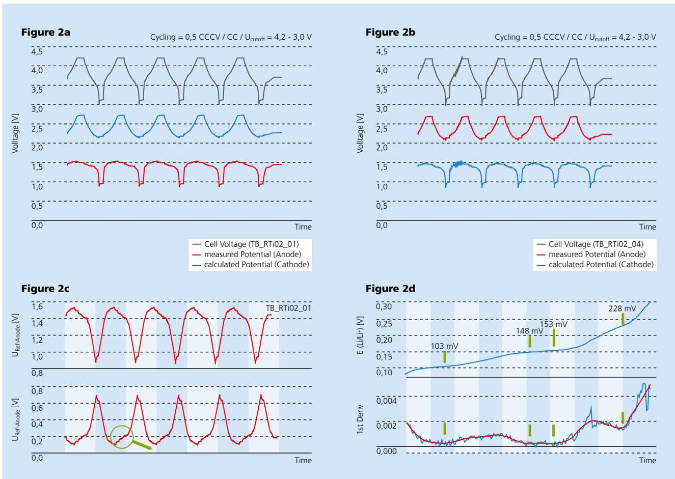
Figure 2: Results of the characterization of a NMC/Graphite cell with an internal reference electrode (LTO)
