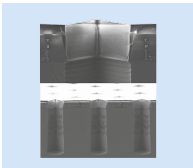
Figure 5: Cross section of the blanking chip with etched apertures close to the CMOS circuit
