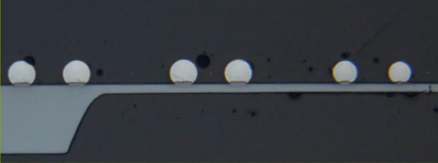
Figure 4: Solder balls applied to 50  $\mu\text{m}$  thin TAIKO wafer. The image shows the thick silicon frame at the wafer periphery
