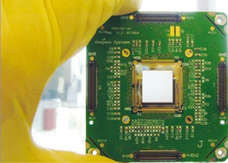
Figure 7: Assembled Deflection Array Plate (DAP)
