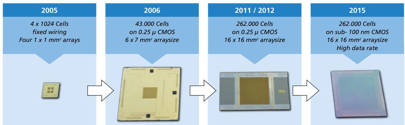
individually addressable electron-beams working in parallel. MBMW is designed to meet the requirements of several upcoming tool generations.
