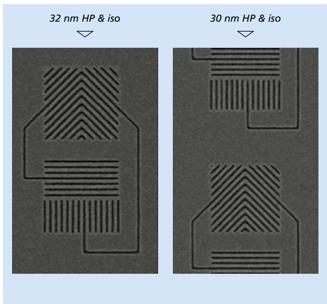
Figure 10: 32/30 nm HP & ISO lines in pCAR (Source: IMS Nanofabrication AG)
