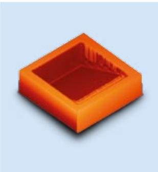
*Figure 3: Interferometric 3D-profile of an inclined slumped window (2.5 x 2.5 cm<sup>2</sup> with an angle of 34°)*
