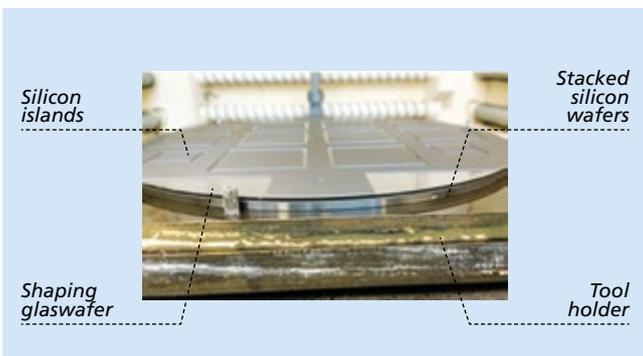
*Figure 2: Wafer stack and vacuum tool forming a reusable mold, with glass wafer on top*
