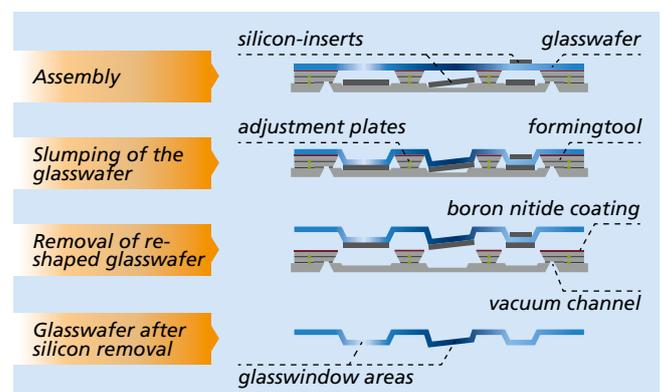
Figure 1: Concept of glass wafer thermoforming process to produce deep cavities with optical windows
