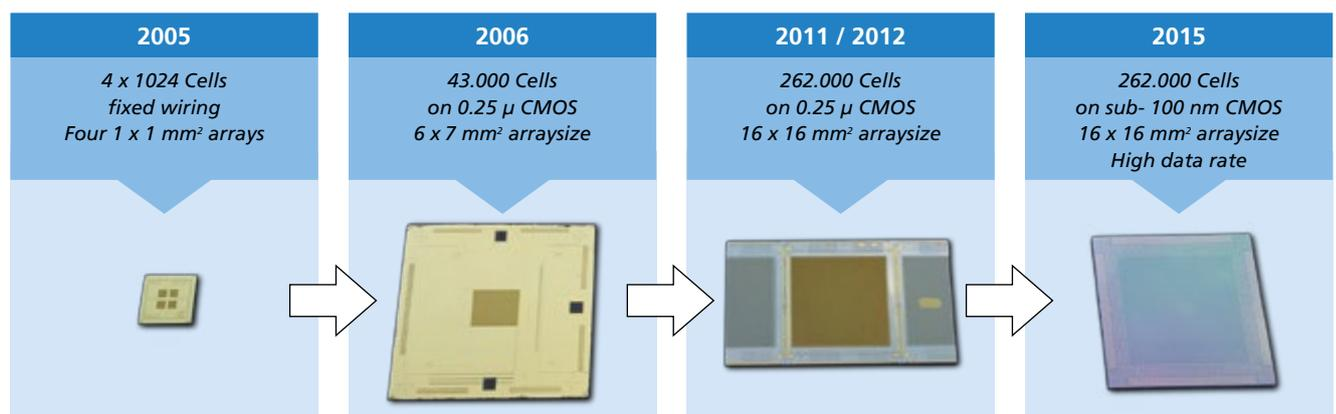
individually addressable electron-beams working in parallel. MBMW is designed to meet the requirements of several upcoming tool generations.
