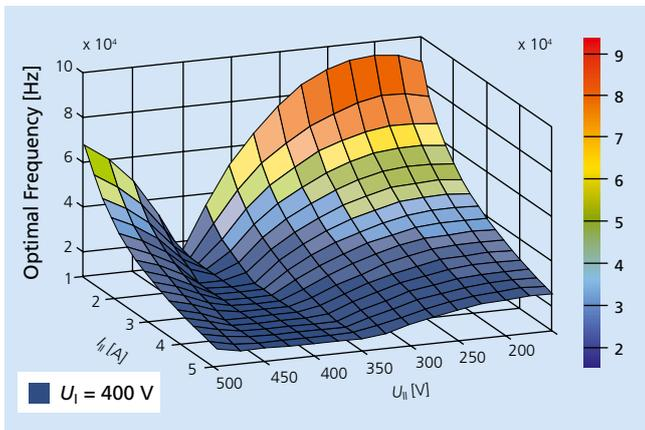
Figure 2: Optimal switching frequency
