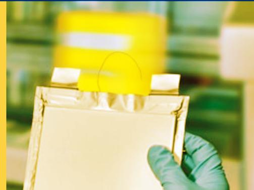
*Lithium polymer cell with integrated temperature sensor*
