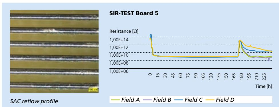
Figure 4: Inline convection reflow soldering. Left: Visual inspection of test board, right: SIR measurement
