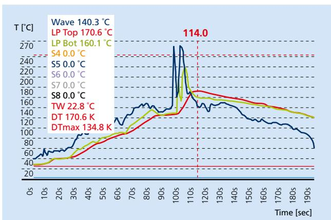
Figure 2: Typical wave soldering profile; max. temperature: PCB Bottom 216°C, PCB Top 171°C
