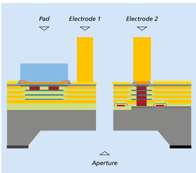
Figure 4: Key MST processes for the blanking plate fabrication
