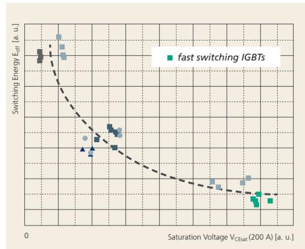
Figure 5: Trade-Off curve for different application specific 200 A Field-Stop IGBTs
