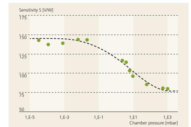
Figure 3: Pirani measurements under vacuum indicate the pixel voltage output as a function of the applied heating power. The detectable vacuum range depends on the pixel design; here the threshold is 1 mbar.
