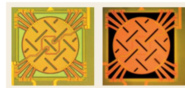
Figure 2: Thermopile pixel with a diameter of approx. 350  $\mu\text{m}$  before and after membrane release etch. The connector line belongs to an integrated Pirani sensor to assess the vacuum level.
