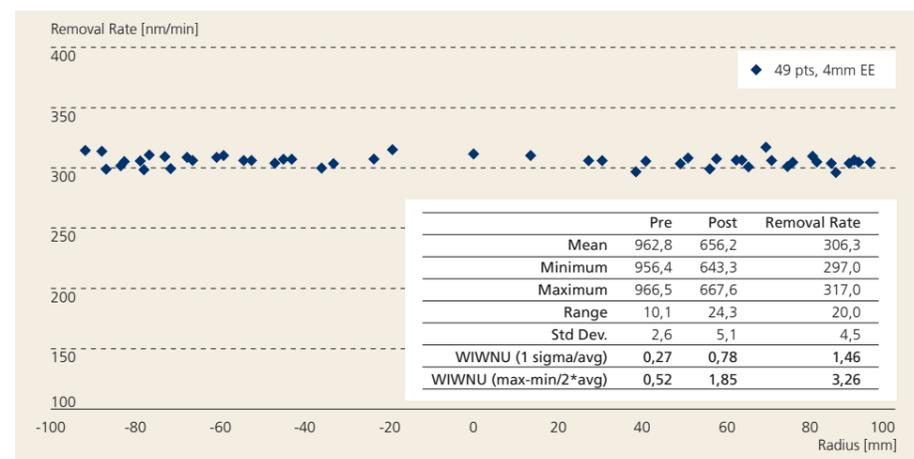
Figure 1: The CMP removal rate on oxide wafers indicates a good uniformity
