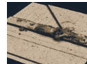
Figure 6: Local damage inspection with 3D laser scanning microscopy
