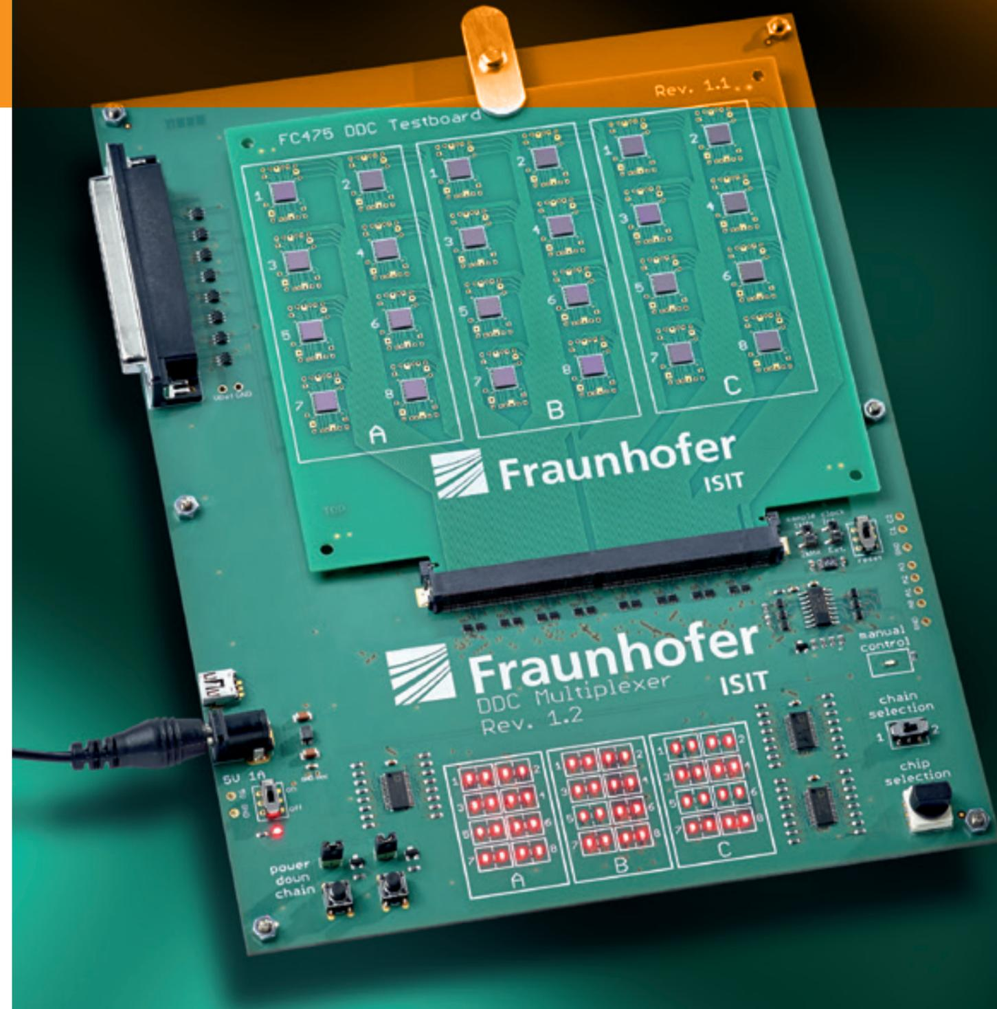
Figure 5: Multiplexing electronics for automated daisy chain measurements
