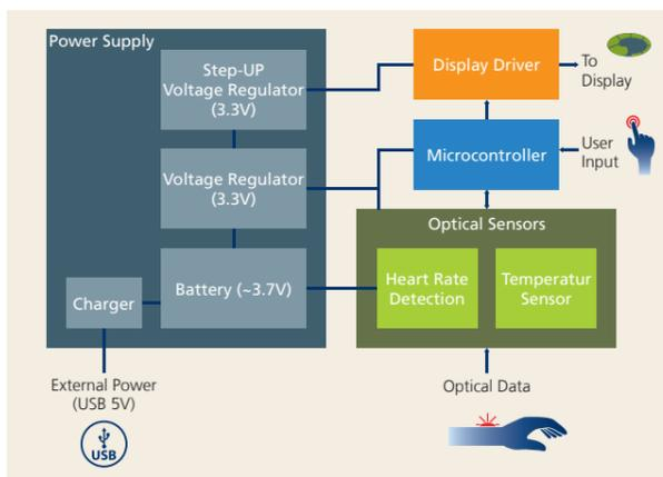
Figure 4: System architecture of the OLED sensor wristband
