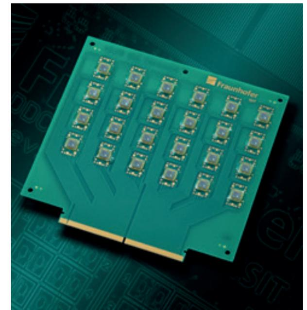
Figure 2: FC475 DDC test-chip evaluation board
