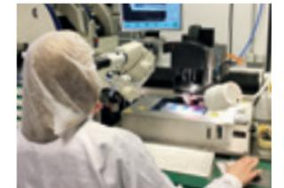
Figure 6: Full automatic wire bonding on panel level
