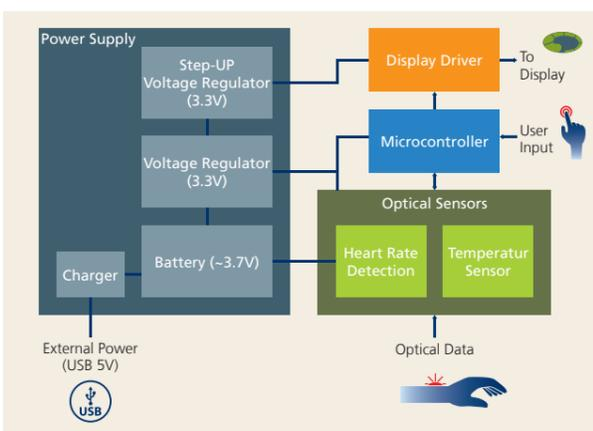
Figure 4: System architecture of the OLED sensor wristband
