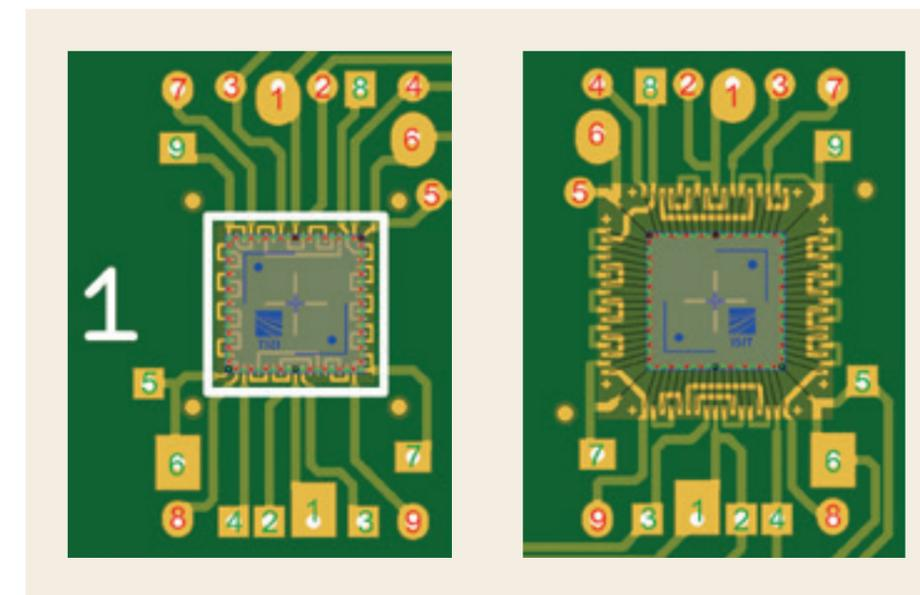
Figure 3: Detailed view of FC475 DDC flip chip and wire bond landing positions
