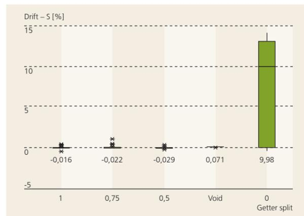
Figure 5: The evolution of cavity pressure in an accelerated 120 hour aging at 150°C was characterized by monitoring the sensitivity drift. Again, the Titanium layer reveals to be an effective means to stabilize the cavity pressure.
