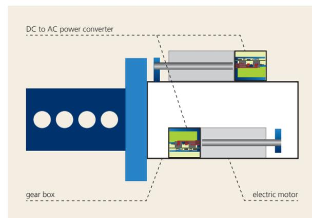
Figure 1: Modular drive concept showing two modular drive units connected to a gear box
