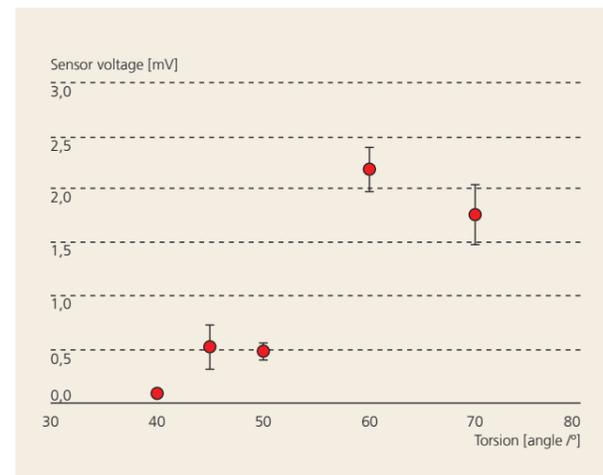
Figure 5: Correlation between sensor voltage and torsion angle. Each point results from five measurements. Values for torsion angles < 40° are buried in noise. Noise may be caused mainly by low sensor sensitivity, pyroelectric effect and friction charging.
