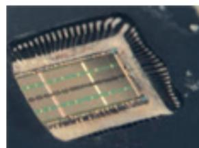
Figure 3: An IC package is etched open for a bond wire inspection
