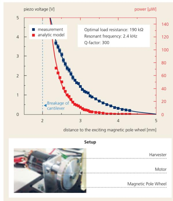
Figure 4: Result of the magnetic pole wheel with the distance of the harvester on the x-axis and the output voltage on the y-axis
