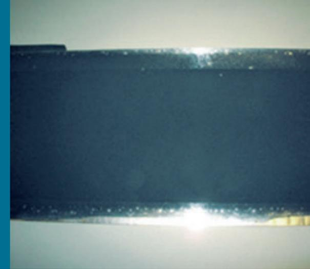
Figure 2: Electrode (cathode) prepared with a water based binder system
