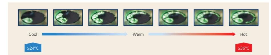
Figure 7: The infrared skin temperature measurement is indicated by the OLED segment display
