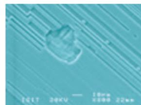
Figure 4: SEM photograph of locally destroyed conductive trace by a sudden current pulse
