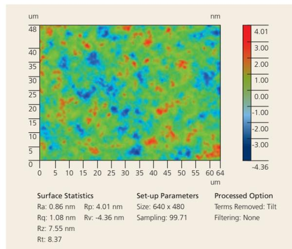
Figure 4: Surface inspection after polysilicon CMP
