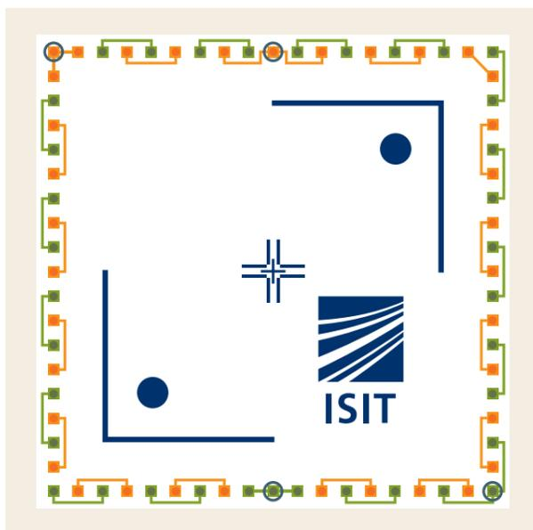
Figure 1: The FC475 DDC test chip with two nested daisy chains (red, green); Kelvin probe contacts are marked by circles
