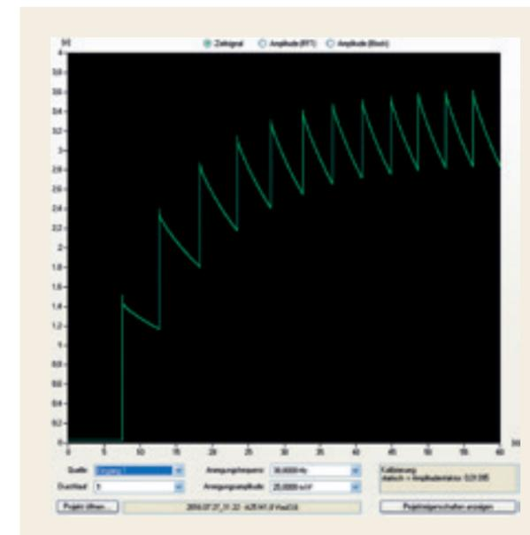
Figure 5: Voltage gradient of the capacitor. Every 5 seconds, an amount of about 0.1 mWs is stored in a 47  $\mu$ F electrolyte capacitor
