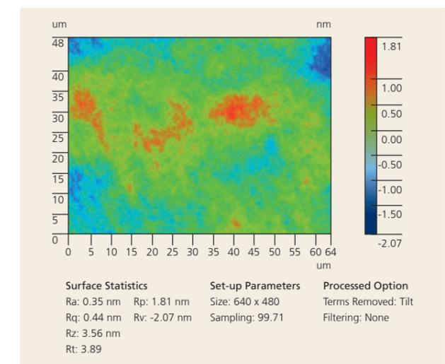
Figure 2: A smooth oxide surface is obtained by CMP
