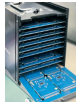
Figure 3: Cartridge module boards after die attach at ISIT
