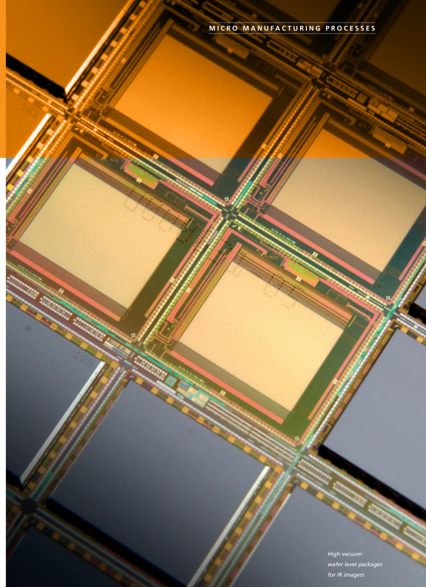
High vacuum wafer level packages for IR imagers
