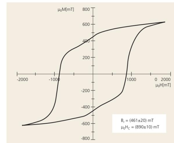
Figure 2: Typical intrinsic demagnetizing curve of the NdFeB micro magnets (particle size 4.5...6.5 μm)
