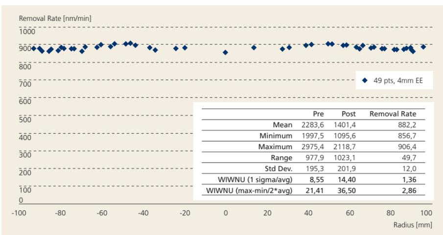
Figure 3: Removal rate and statistics on epitaxial polysilicon
