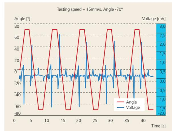
Figure 4: Voltage over time graph (torsion setup, planarized cleanroom cloth substrate)
