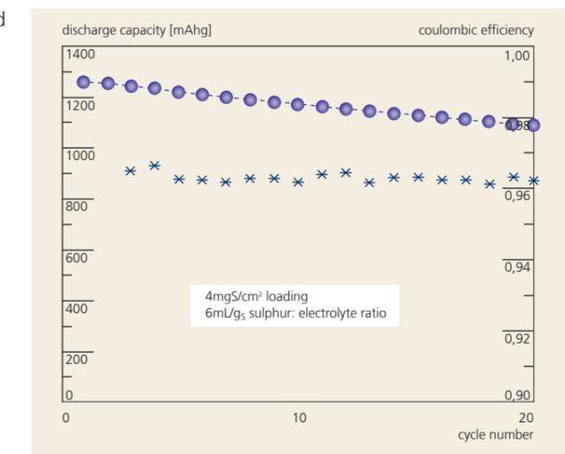
Figure 3: Cycle stability of Li-S cells using a cathode developed by Fraunhofer ISIT
