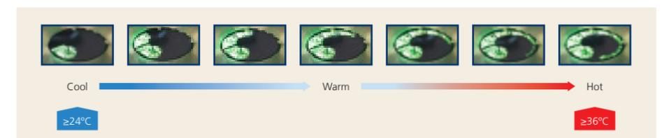
Figure 7: The infrared skin temperature measurement is indicated by the OLED segment display
