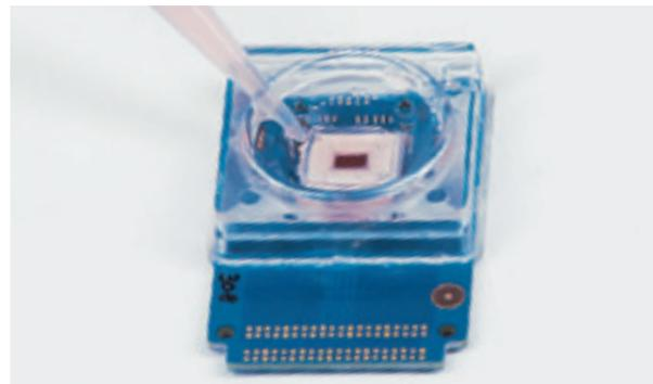
Figure 2: A precision molded second plastic cap with a fluidic window opening protects the sensitive chip area and defines a cell cultivation well
