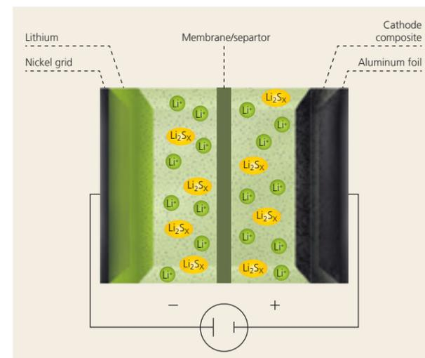
Figure 1: Schematic view of Li-S cell with polysulphide shuttle mechanism
