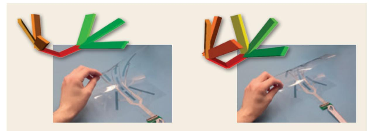
Figure 2: Signal visualization of a bent torsion sensor on PET for elbow measurement
