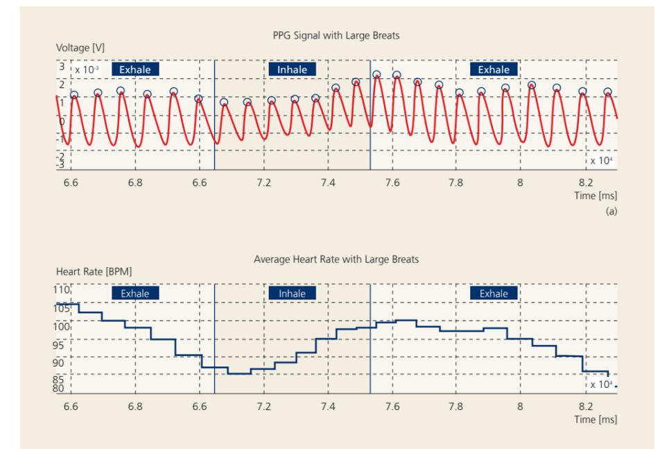
Figure 6: HR measurements through optical sensing. Upper graph: Pulse frequency. Lower graph: Heart rate in correlation with the breathing activity.
