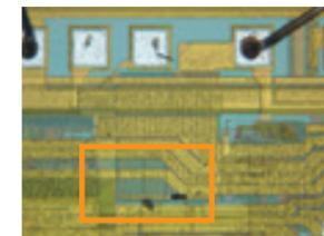
Figure 5: EOS damage, overview with light microscopy (50x)
