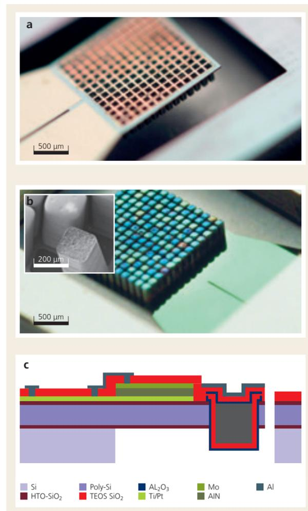
Figure 1: Magnetic energy harvester device from the front (a) and from the rear side (b). The inset depicts a SEM-image of a micro magnet. The whole structure consists of 13x 13 micro magnets. (c) Cross section drawing of the device.
