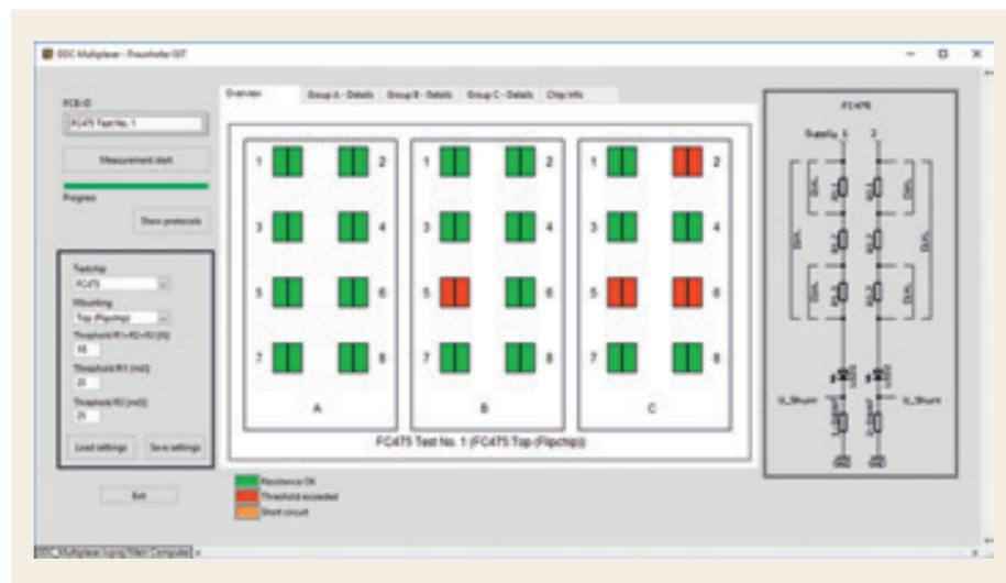
Figure 4: Based on user defined thresholds the overview page of the measurement software indicates good and bad chips as well as short circuits graphically. Detailed measurement results can be obtained from the "Group A/B/C - Details" pages not shown in the image.
