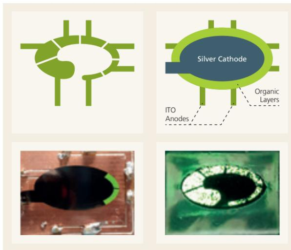
Figure 3: OLED display design for health parameter indication and visualization. Upper left: Structured ITO anode. Upper right: Display structure. Lower left: Two segments addressed directly after fabrication. Lower right: All segments addressed, degradation (mainly the ITO anode) after three months.
