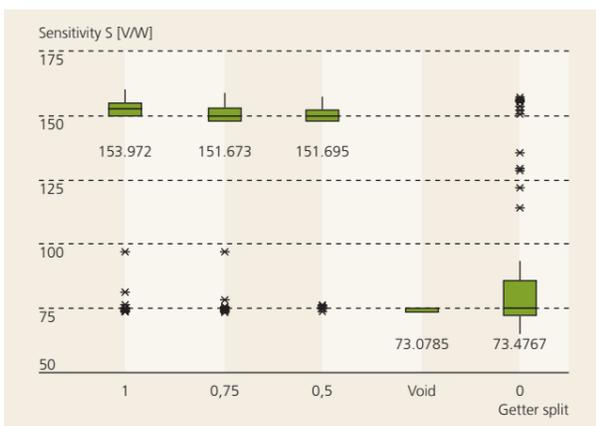
Figure 4: The gettering effect of the Titanium aperture was studied on 3000 dies from 5 wafers with different getter area. In the box plot, all getter shapes have a narrow standard deviation of the Pirani sensitivity while the getter-free package is unable to maintain the vacuum.
