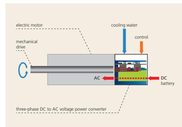
Figure 2: Modular drive unit with 40 kW power
