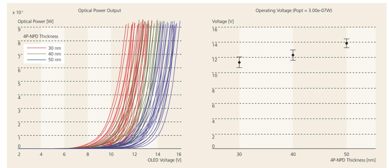
Figure 2: (left) Optical power output depending on OLED voltage. (right) Voltage as a function of the layer thickness
