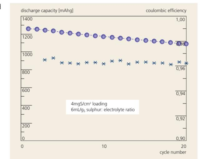
Figure 3: Cycle stability of Li-S cells using a cathode developed by Fraunhofer ISIT
