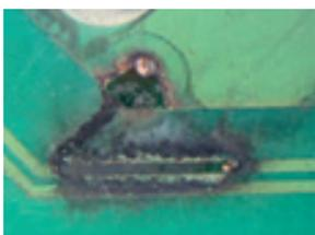
Figure 9: Burnt track on PCB after corrosion
