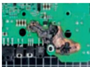
Figure 1: Photograph of an assembled board with a fire-damaged area in the lower right
