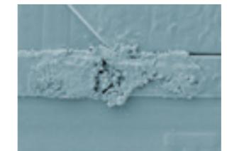
Figure 7: Local damage inspection with SEM. Obviously the conductor is molten
