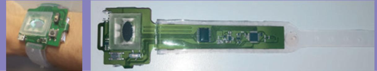
Figure 5: OLED wristband with integrated optical sensors for heart rate and temperature measurement
