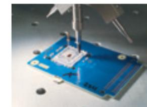
Figure 5: The first plastic cap with its fluidic window is aligned and placed above the sensor chip
