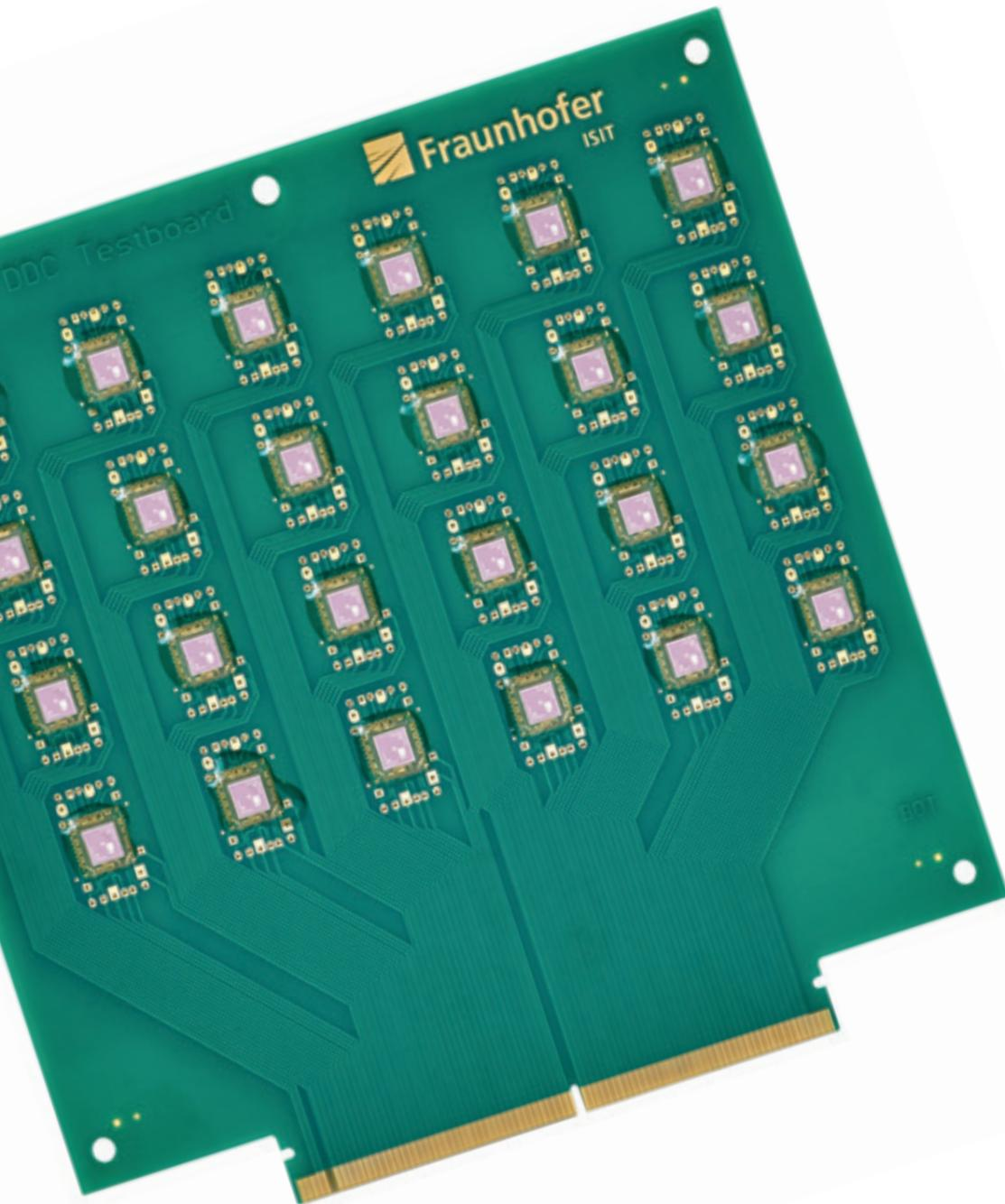
Customer specific test substrate for adhesive screening
