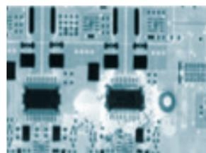
Figure 2: 2D X-ray analysis of a locally burnt board (white area)
