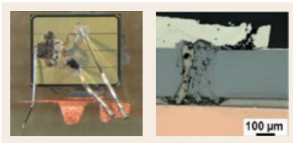
Figure 8: Damage of a silicon power transistor (left) with partial delamination (right) after EOS
