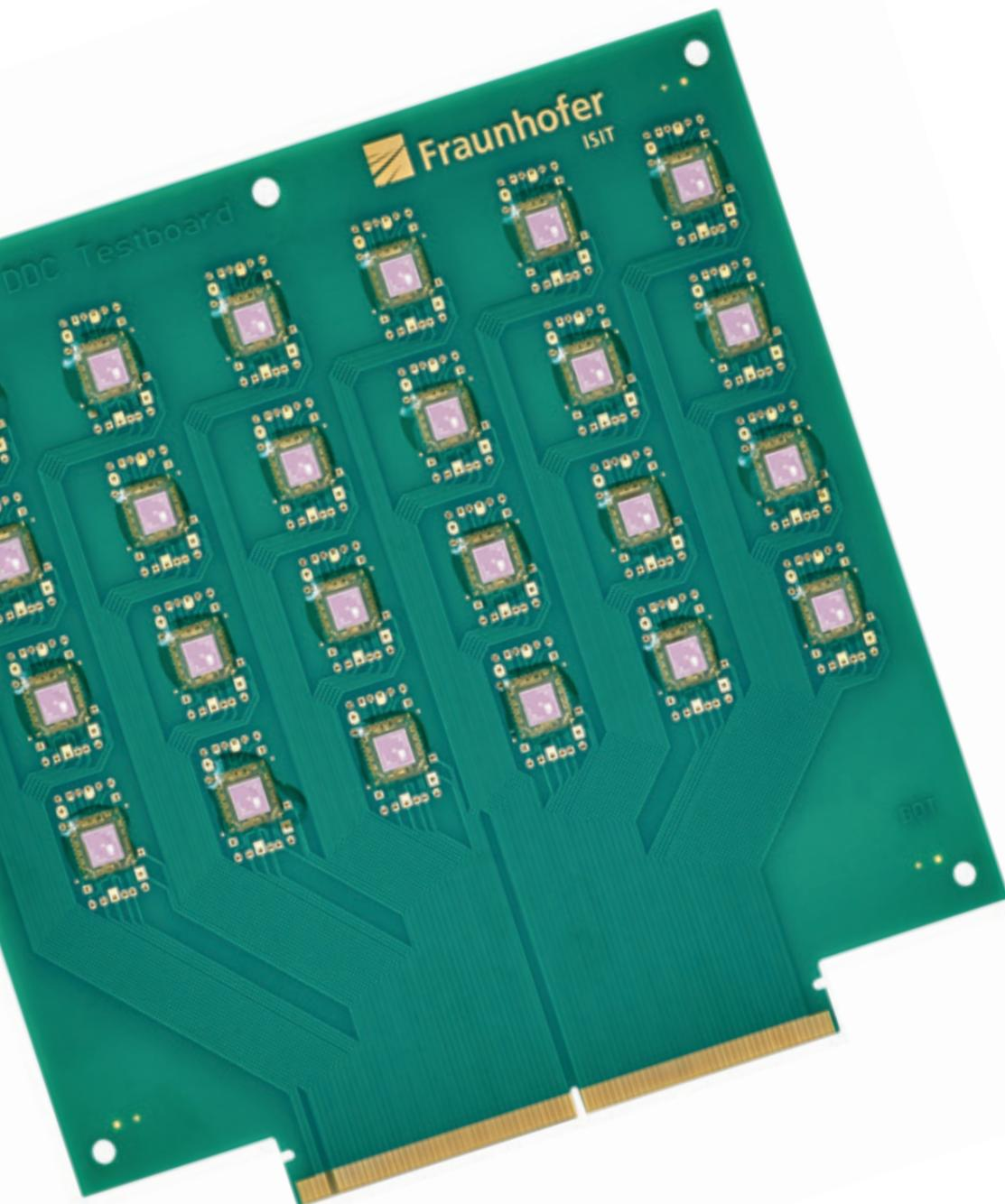
Customer specific test substrate for adhesive screening
