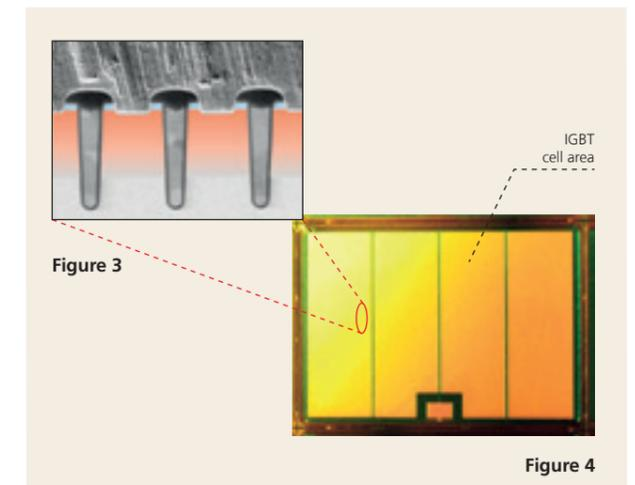
Figure 3: Cross section of a standard trench IGBT
