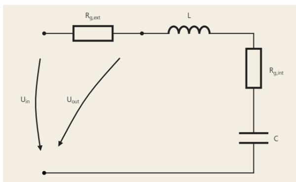
Figure 1: Equivalent circuit of an IGBT gate branch
