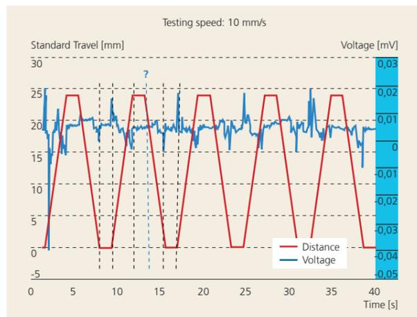
Figure 3: Voltage-time characteristics (bending test, planarized cleanroom cloth substrate). Some signals are obviously below the signal noise level (indicated by a “?”)
