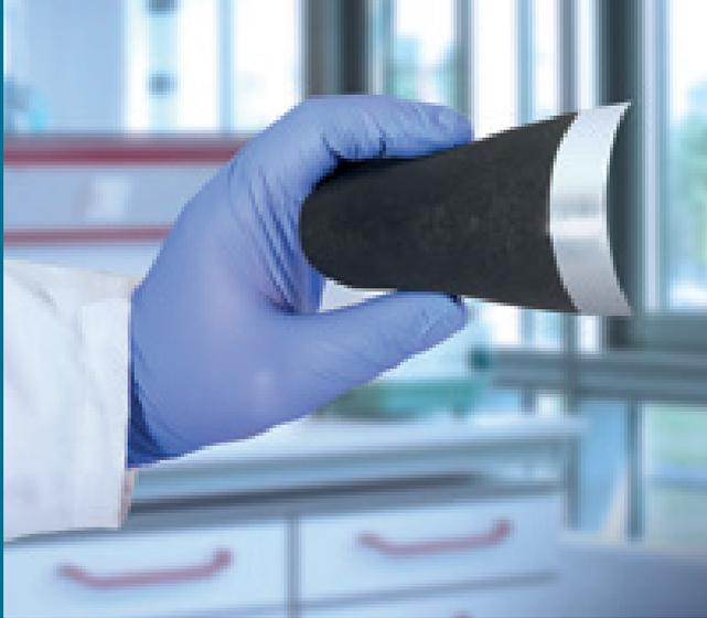
Figure 2: Picture of a dry coated electrode
