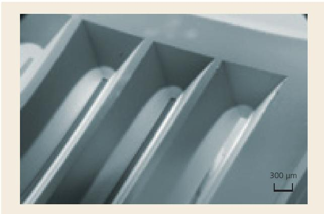
Figure 2: SEM picture of Silicon electrodes after diamond coating at Condias
