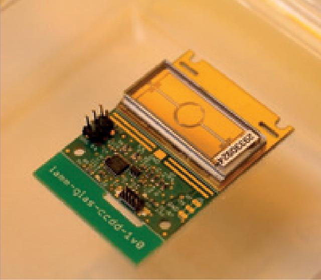
Figure 2: Circuit board with a large-aperture scanning system
