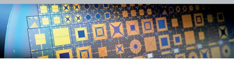
1 Variety of piezoelectric MEMS devices for acoustic applications on an 8-inch wafer.
