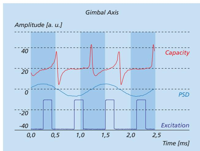
Figure 4: Measured signal waveforms
