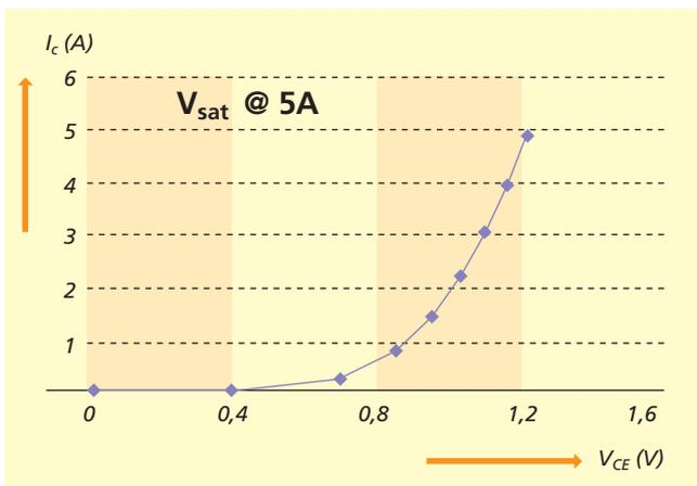
Figure 7: IGBT collector-emitter voltage ( $V_{ce}$  (V)) of 1,2 V measured at 5 A on wafer level
