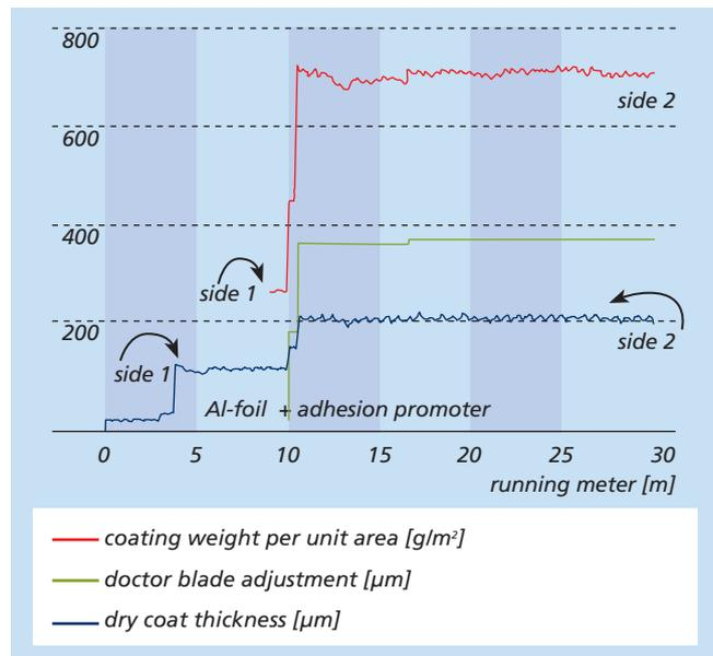
Figure 5: Coating result of a double-sided coating with a NMP based test slurry. The data from the inline sensors show the profiles along the length of the electrode foil
