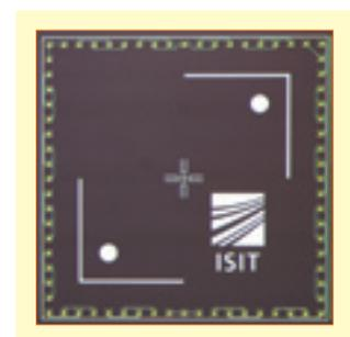
Figure 6: New testchip Design FC 475 DDC with two interlaced daisy chains
