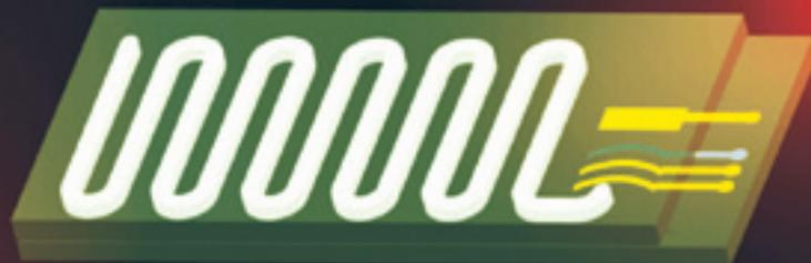
Figure 1: Construction scheme of chromatography chip
