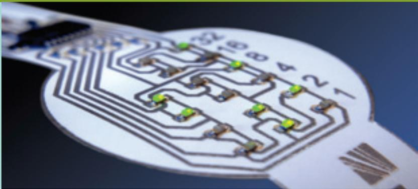
*Printed functional structures on paper: binary clock*
