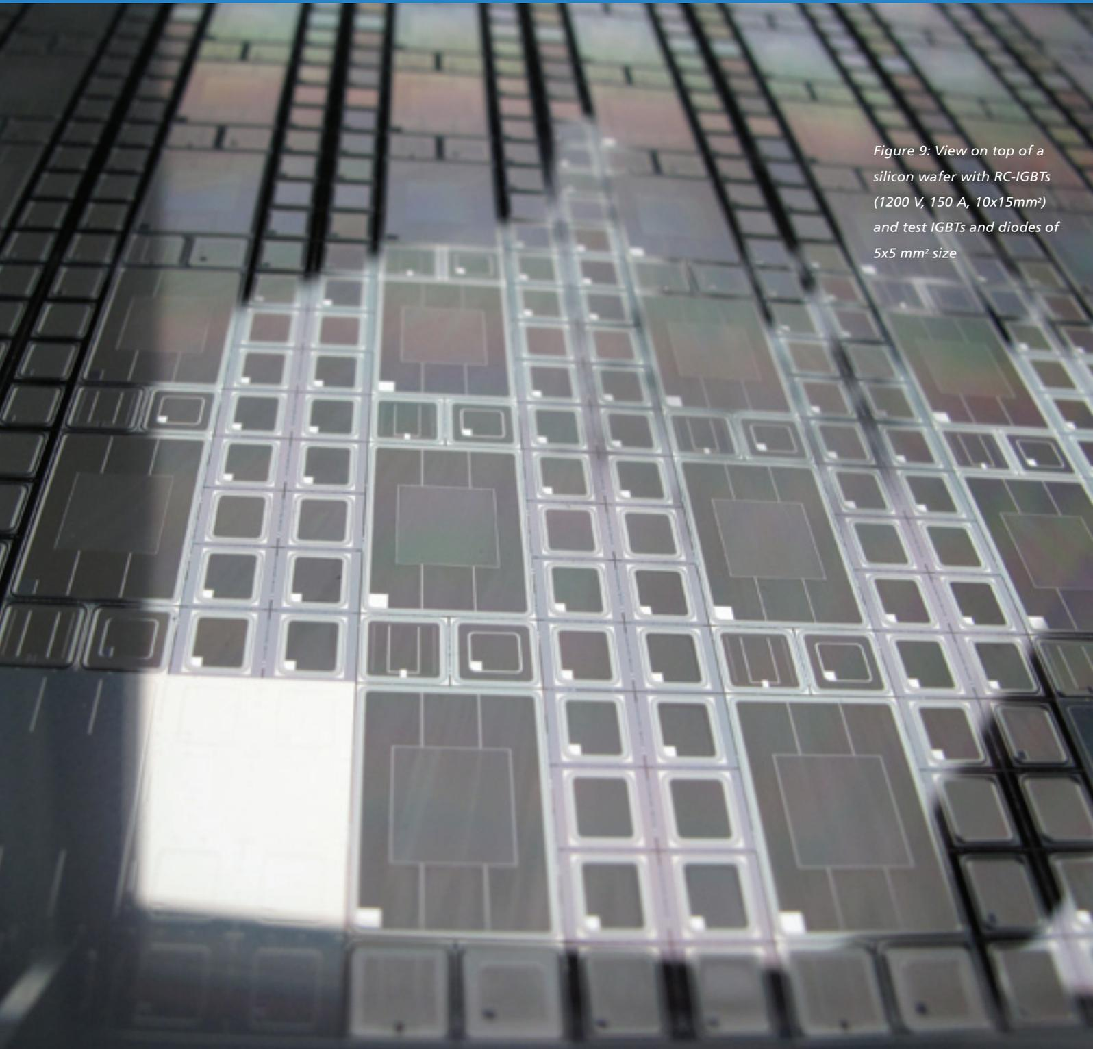
*Figure 9: View on top of a silicon wafer with RC-IGBTs (1200 V, 150 A, 10x15mm<sup>2</sup>) and test IGBTs and diodes of 5x5 mm<sup>2</sup> size*
