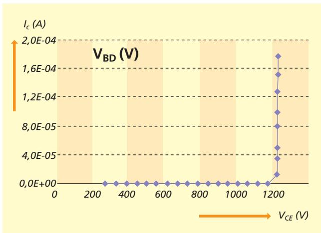
Figure 6: Break down voltage measurement ( $I_c$  vs.  $V_{ce}$  for 1200 V IGBT)
