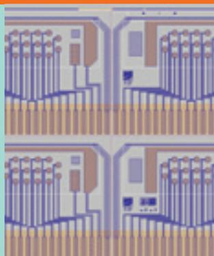
*Silicon based electrical array biochips*
