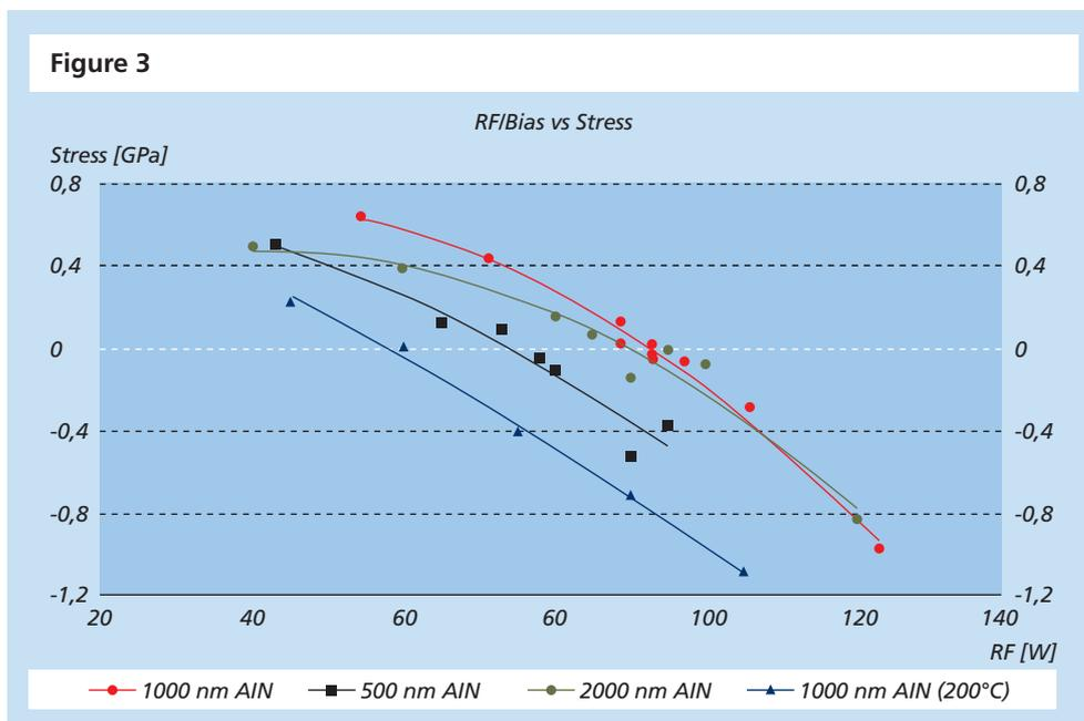
Figure 3: Dependence of the mechanical stress in the sputtered AlN films from the applied RF power. To achieve zero stress, the power level must be adapted to the projected film thickness. Using a process temperature of 200 °C instead of 400 °C used in the standard process leads to a drastical shift in the mechanical stress behavior of the deposited AlN films (lower vs. upper curve)
