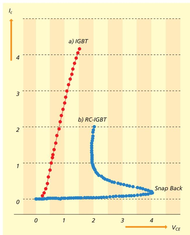
Figure 2: Simulation of the snapback characteristic
