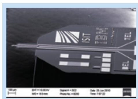
Figure 11: SEM picture of the complete AFM cantilever chip
