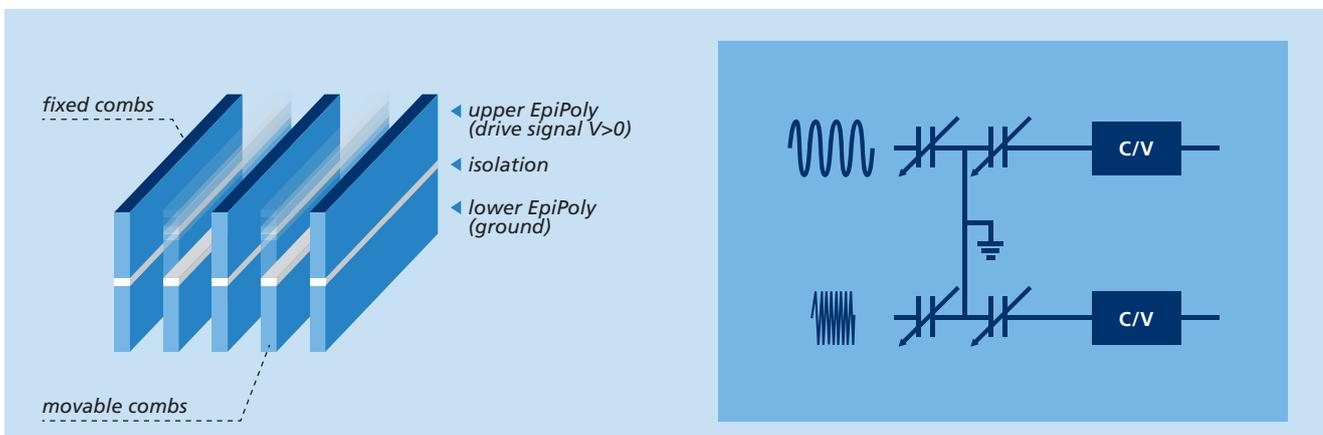
Figure 3: Comb structure for electrostatic driving and capacitive detection (left) and the corresponding electrical diagram including clv-converters (right)
