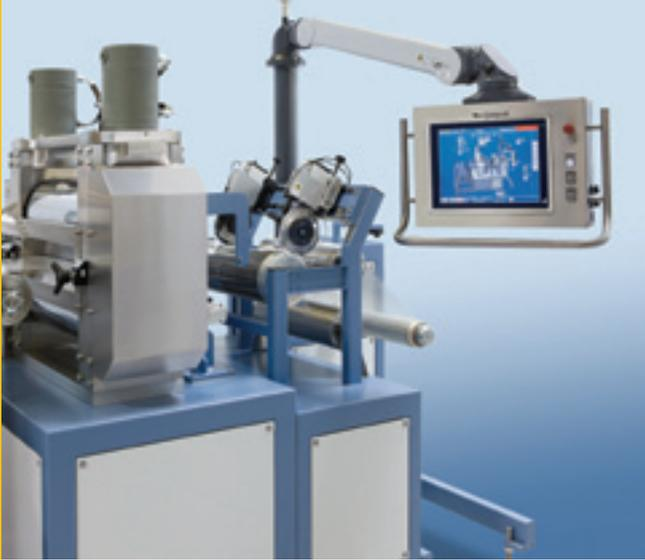
Figure 4: Final inline foil processing (after the drying stretch) consisting of calendaring unit, dry coat thickness sensor and edge cutting tool
