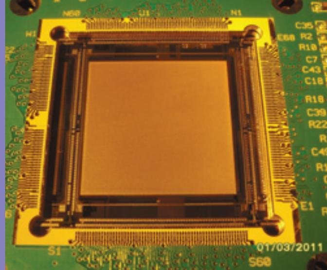
*Vacuum packaged two-axis-scanning micromirrors with inclined optical glass windows*
