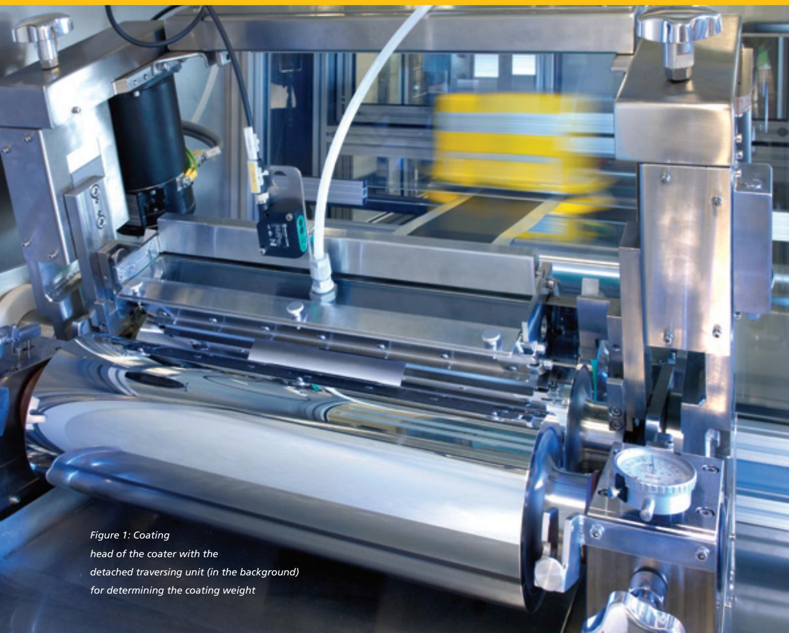
*Figure 1: Coating head of the coater with the detached traversing unit (in the background) for determining the coating weight*
