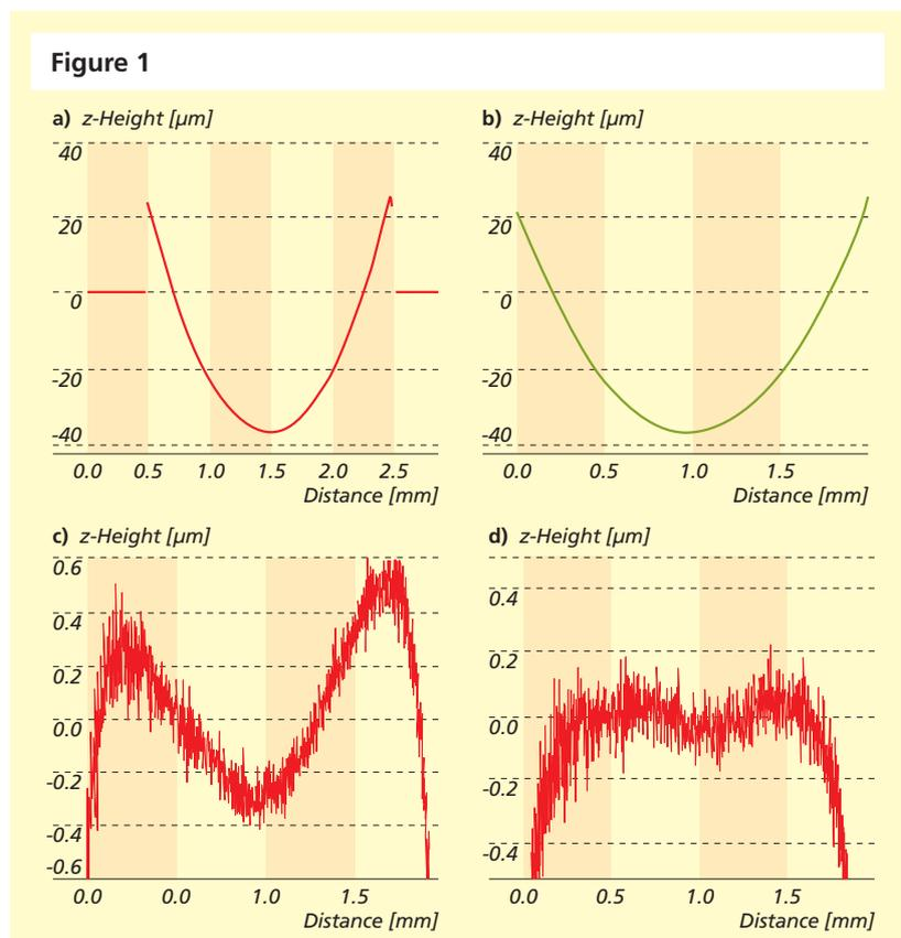
Figure 1: Measured curvature of a lens made of Borofloat® 33 (a); scanned surface of the lens (b); deviation from the spherical contour without any edge exclusion (c); deviation of the lens form with 15% edge exclusion (d)
