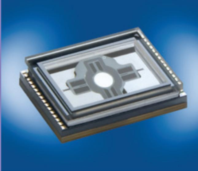
Figure 1: Vacuum packaged 2D MEMS scanning mirror; the chip volume is only 0.07 ccm
