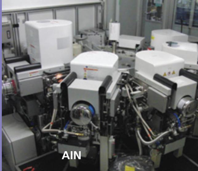
Figure 2: Rear side of the cluster line. Around the central handling robot, the various process chambers can be seen. The lower left chamber is used for sputtering AlN
