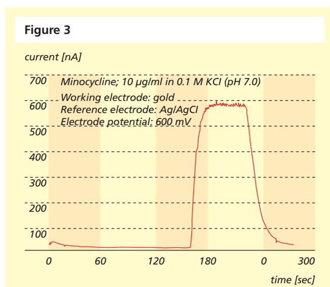
*Figure 3: Amperometric signal of the antibiotic minocycline on gold electrode*
