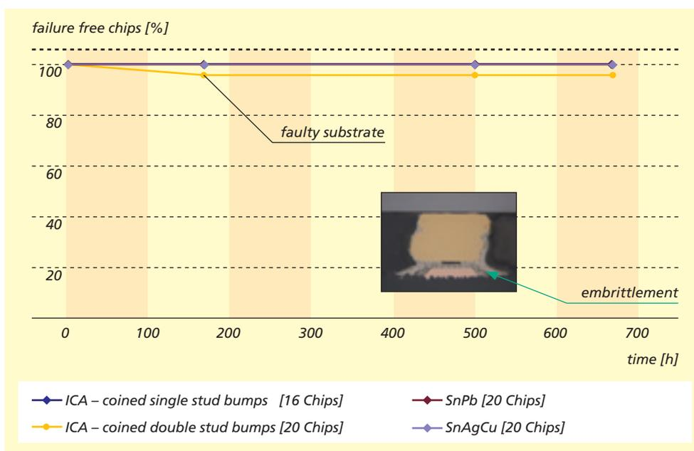
Figure 5: Heat and humidity test results (85 °C / 85 % rel. hum.) for isotropic conductive adhesive (ICA) and solder bumps
