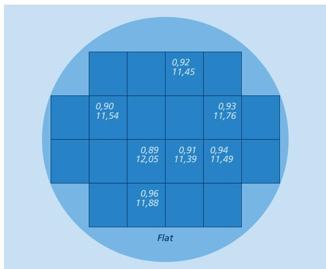
Figure 9: Results of electrical and piezoelectrical characterization of the AlN test wafer from Fig. 8. The  $e_{31,f}$  coefficients (upper value) are in the range of 0.89...0.94 C/m<sup>2</sup>, while the permeability (lower value) ranged from 11 to 12
