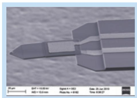
Figure 12: Detail of AFM cantilever with integrated AlN structure and tip
