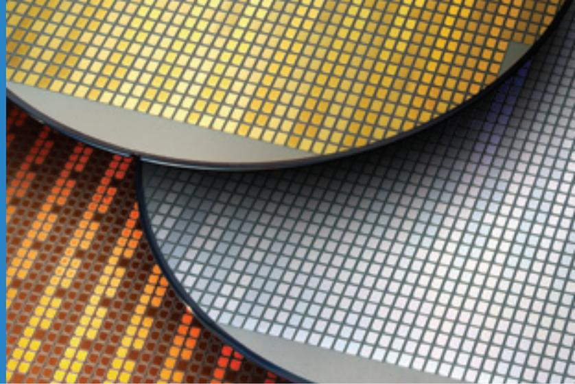
*IGBTs with customer-specific metallization (standard Al, electroless Ni/Au and Cu-metallization) for advanced assembly techniques*
