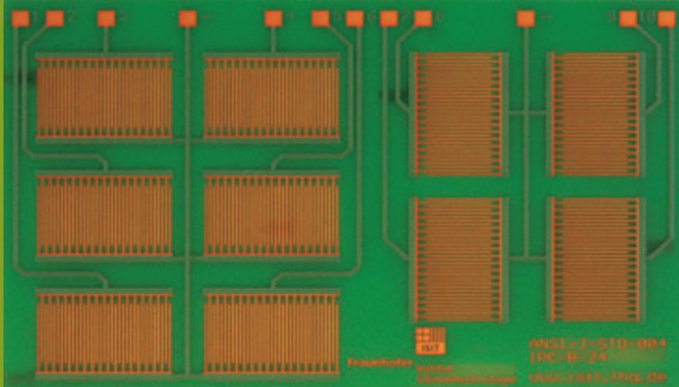
Figure 1: ISIT test board with 10 comb patterns for SIR-measurements
