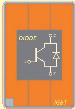
Figure 1: Layout of an RC-IGBT with integrated diode (dark) and IGBT trench cells (orange)
