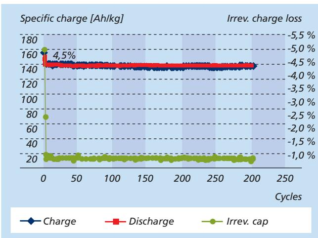
Figure 6: Test cell characteristics of a half-cell with a  $\text{Li}_4\text{Ti}_5\text{O}_{12}$  anode foil from the new coating facility showing good cycle stability at 1C (100 % DOD)
