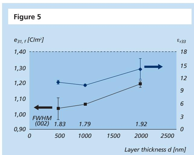
Figure 5: Measured  $e_{31,f}$  values for AlN layers of different thicknesses. Thin AlN layers showed a decrease in their piezoelectric performances
