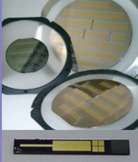
Figure 6: Wafer with test pattern for the characterization of the piezoelectric performance of sputtered AlN films. The inset picture shows a diced test chip used for determining the  $e_{31,f}$  values of the piezoelectric film
