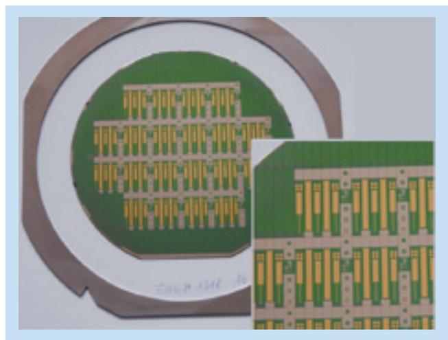
Figure 8: Test wafer with AlN test structures processed on the carrier wafer with glass pins. Underneath the AlN layer, platinum as the bottom electrode was applied
