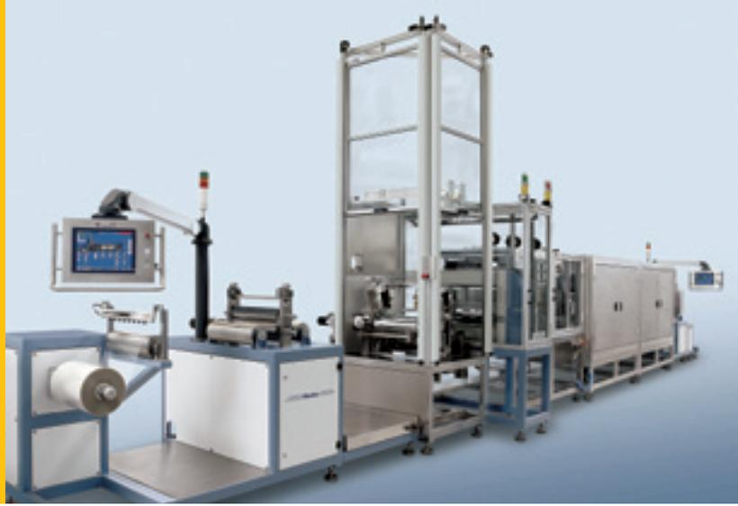
Figure 2: A full view of the coating facility for electrode and separator foils
