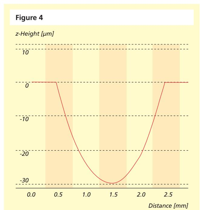
Figure 4: Scan over a lens surface made of Glass II. The central cut through the lens is visualised
