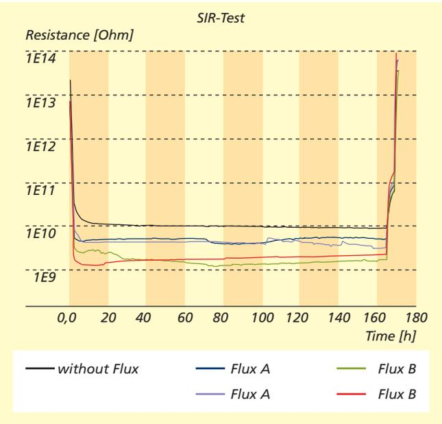
Figure 2: Diagram with test data for two different fluxes. Higher resistances at the beginning and at the end of test because of lower humidity in the climate chamber
