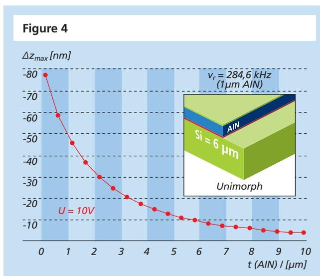
Figure 4: FEM simulation of cantilever deflection for a given applied voltage of 10 V as a function of AlN layer thickness. Using thinner AlN films would increase the achievable beam deflections
