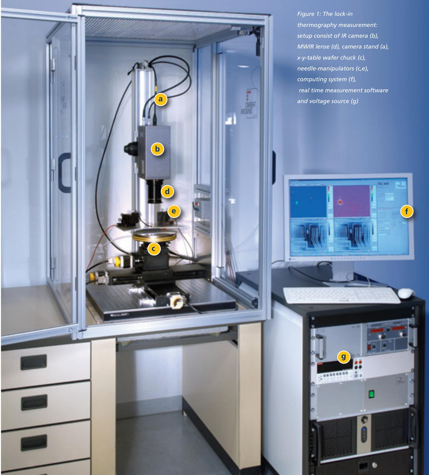
Figure 1: The lock-in thermography measurement: setup consist of IR camera (b), MWIR lens (d), camera stand (a), x-y-table wafer chuck (c), needle-manipulators (c,e), computing system (f), real time measurement software and voltage source (g)
