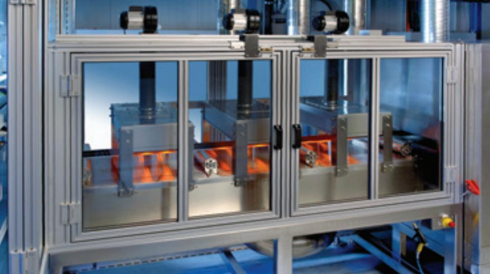
*Figure 3: Inline infrared unit for preliminary drying of coated foil strip*
