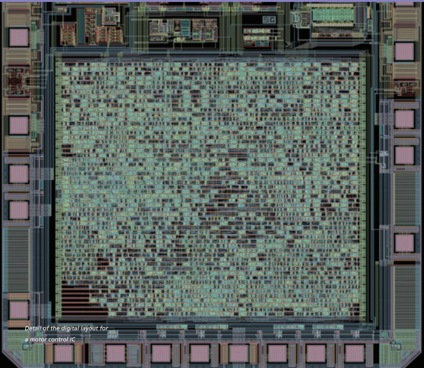
*Detail of the digital layout for a motor control IC*
