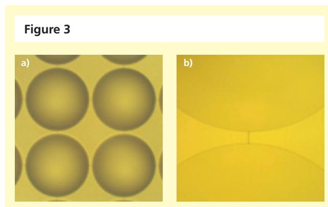
Figure 3: Microscopic view (2.5X) of a part of a lens wafer (left side). In this experiment the lenses are made of „Glass II“. On the right side, a more detailed view is visible (20X). In both pictures all lens surfaces are completely free of glass defects.
