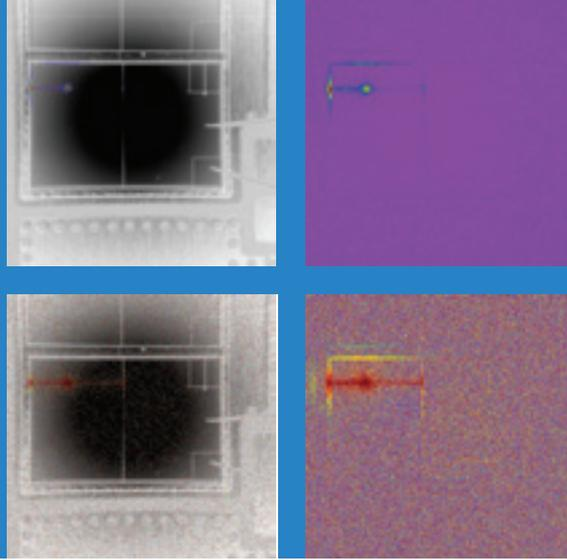
Figure 2: Hot spot detection with lock-in IR thermography: Amplitude and Phase pictures of a power transistor with gate leakage
