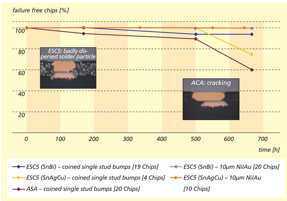
Figure 4: Heat and humidity test results (85 °C / 85 % rel. hum.) for ESC5 and ACA
