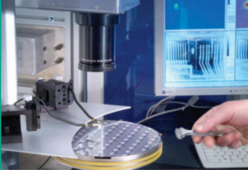
*Micro lock-in thermography measurement system for defect localization*
