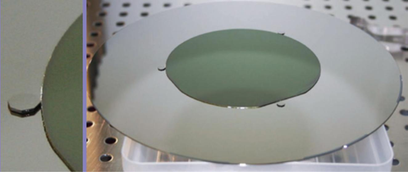
Figure 7: The 200 mm carrier wafer features small additional glass pins to guarantee a fixation of the 100 mm device wafer. Since the silicon surface of the carrier wafer remains unprocessed, a very smooth and even contact area between the silicon wafers can be achieved. The glass pins are thermally adapted to silicon and bonded anodically to the silicon wafer. An additional metal layer ensures good electrical coupling and homogeneous temperature rise during thermal ramp-up
