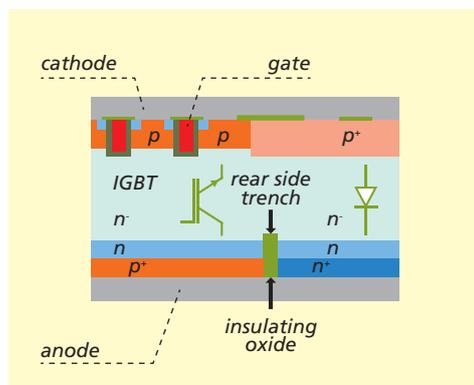
Left, Figure 3: Cross section of through the silicon trench insulation (green) between Diode and IGBT
