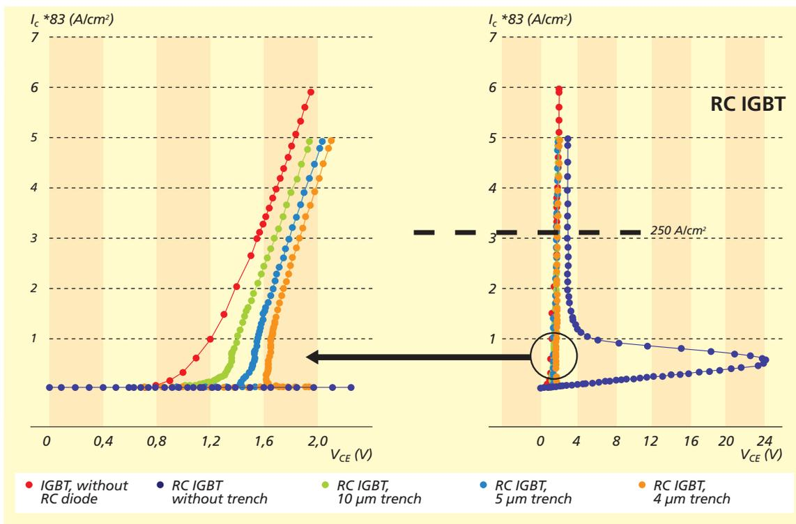
Figure 5: Snapback progression of RC-IGBT with increasing depth of the rear side trench of 4 μm to 10 μm. The rear side trench strongly reduces the snapback effect
