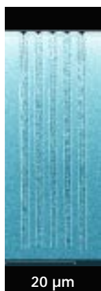
Figure 4: Filling of 60 μm deep and 2 μm wide trenches with poly-silicon.
