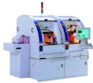
Figure 8: Flip chip die bonder for ultra-thin silicon (Datacon 2200 apm).
