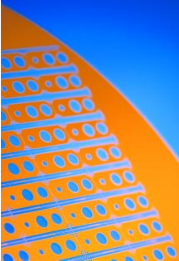
Devices for UV-laser ablation and polishing the cornea surfaces of human eyes.
