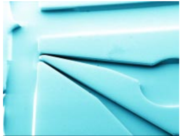
Figure 1: Microfluidic channel structures in borosilicate glass: substrate with step height of 150\ \mu\text{m} and minimum channel width of 20\ \mu\text{m} .
