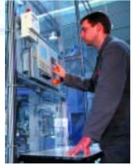
Lithium polymer battery production line – control of electrolyte dispenser unit.
