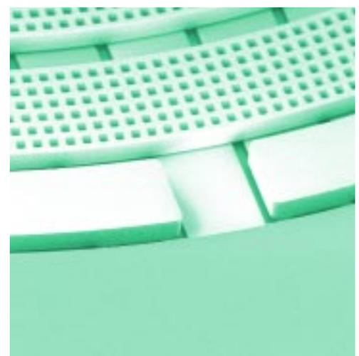
Microsensor structure for inertial measurements.
