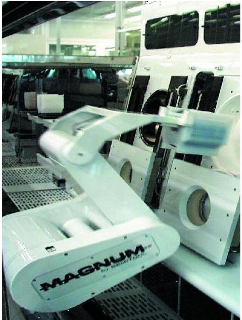
Wafer loading into a Semitool spray clean tool.
