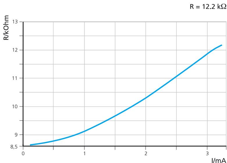
Figure 9: Resistance characteristic ( $R/\Omega$  vs  $I/A$ ) for the TiN lines. Reversibility is given until  $R = 12.2 \text{ k}\Omega$  according to  $T = 600^\circ \text{C}$ .
