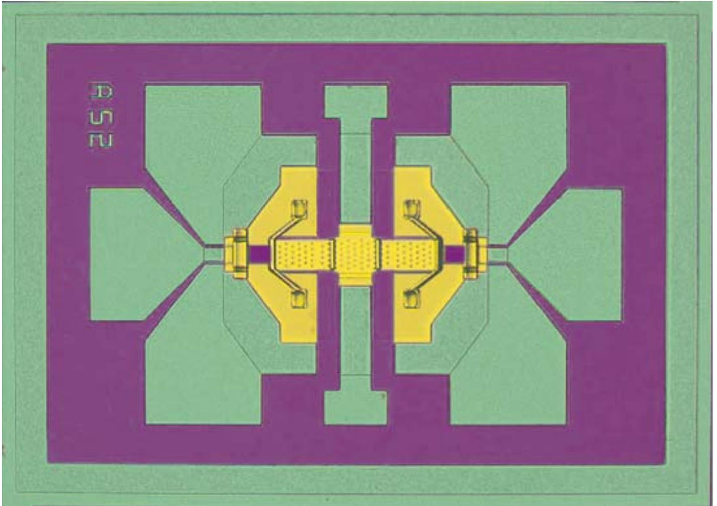
operation without charge induced sticking of the membrane using unipolar DC voltages only. Up to now, total on times of more than 1500 hours without failure have been demonstrated. The on-capacitance of switches with a typical AlN thickness of 300 nm is in the range of 160-180 pF/mm<sup>2</sup>. For air gaps of 2-3 μm between membrane and signal line on-off ratios in the range of 15-30 can be expected.
