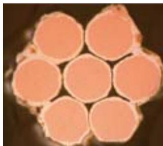
Figure 11: SnAgCu 0.5 – strong dissolution 1000x.
