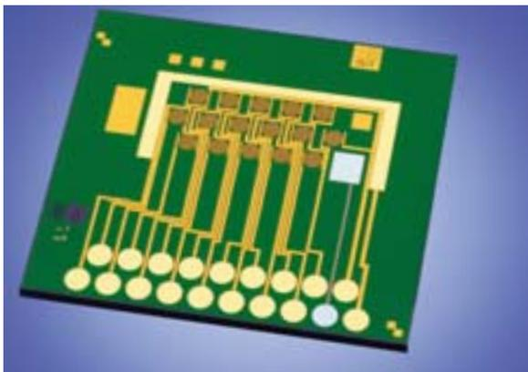
Electrical Silicon biochip with integrated reference electrode.
