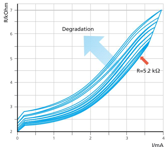
Figure 5: Resistance characteristic ( $R/\Omega$  vs  $I/A$ ) for the Ti/TiN lines. The endpoint of the imposed voltage is stepwise increased from 21 to 30 V. The scaling on the I-axis is from 3.9  $\mu$ A to 4.0 mA. Reversibility is given until  $R = 5.2$  k $\Omega$  according to  $T = 380$  °C.
