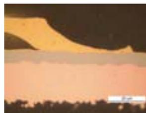
Figure 8: Wedge side of the wire.
