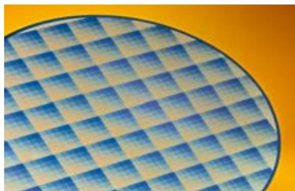
200 mm CMP test wafer.
