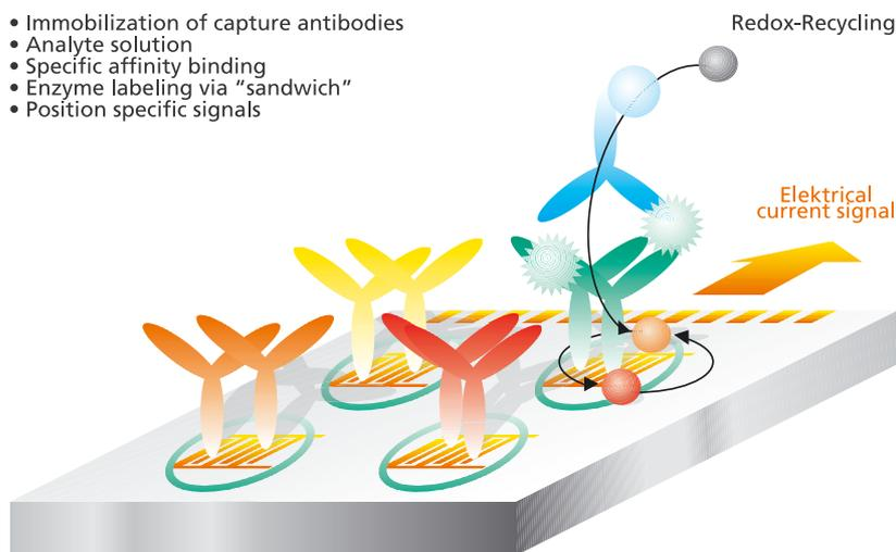
Figure 1: Scheme of a sandwich assay procedure.
