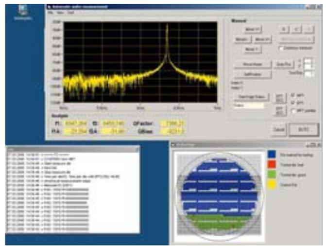
Figure 6: Graphical User Interface of the automatic wafer endtest.
