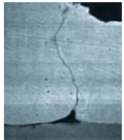
Figure 9: SEM image of wedge bond with crack.
