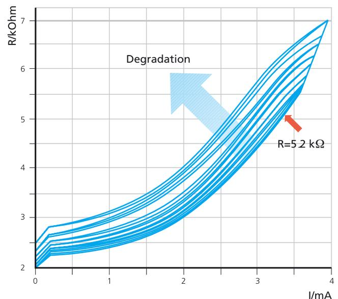
Figure 5: Resistance characteristic ( $R/\Omega$  vs  $I/A$ ) for the Ti/TiN lines. The endpoint of the imposed voltage is stepwise increased from 21 to 30 V. The scaling on the I-axis is from 3.9  $\mu$ A to 4.0 mA. Reversibility is given until  $R = 5.2$  k $\Omega$  according to  $T = 380$  °C.
