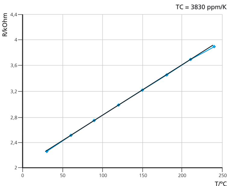
Figure 4: TC measurement of a Ti/TiN resistance.
