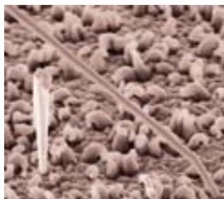
Figure 14: Microsection of tin layer with grown whisker (preparation plane measured with optical measuring station).
