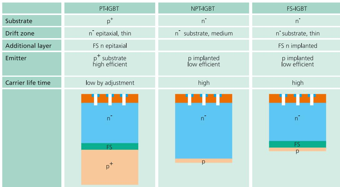
Figure 1: Overview on different Trench IGBT concepts.
