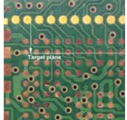
Figure 2: Printed Circuit Board with visible target, a row of microvias.
