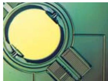
Two axis micro mirror developed for laser projection applications.
