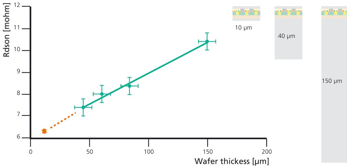
Figure 2: Dependence of On-resistance  $R_{Dson}$  vs substrate thickness for 30 V Trench PowerMOS devices.
