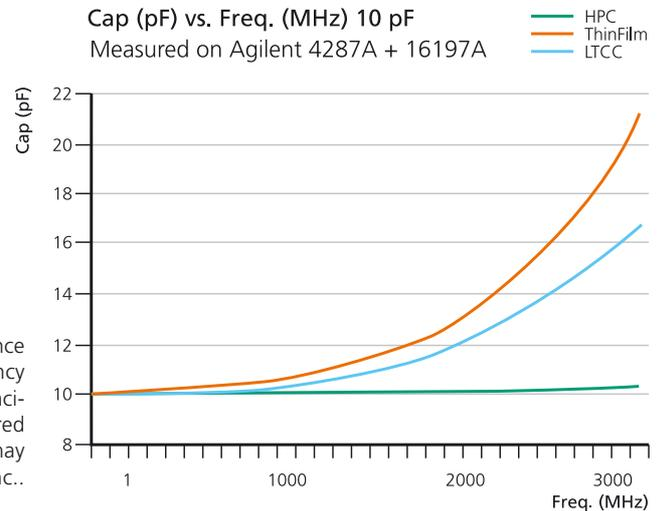
parasitics could be realised by the use of the special SMD component designs and the employing of a solder bump technique. Typically, the RF capacitance value of standard components is increasing with frequency due to parasitic inductance impact. As can be seen in figure 4 there is nearly no capacitor change with increasing frequency which is a special advantage for this circuit design.
