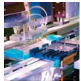
Assembly of Lithium polymer battery stacks.
