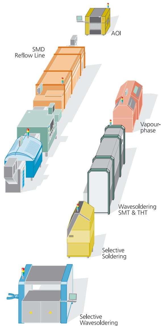
Figure 1: Schematic of the training line set-up.
