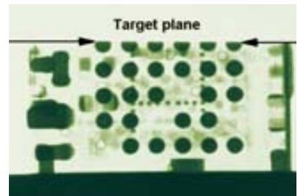
Figure 3: Radiographic image of hidden target, a row of solder balls on a CSP-component.
