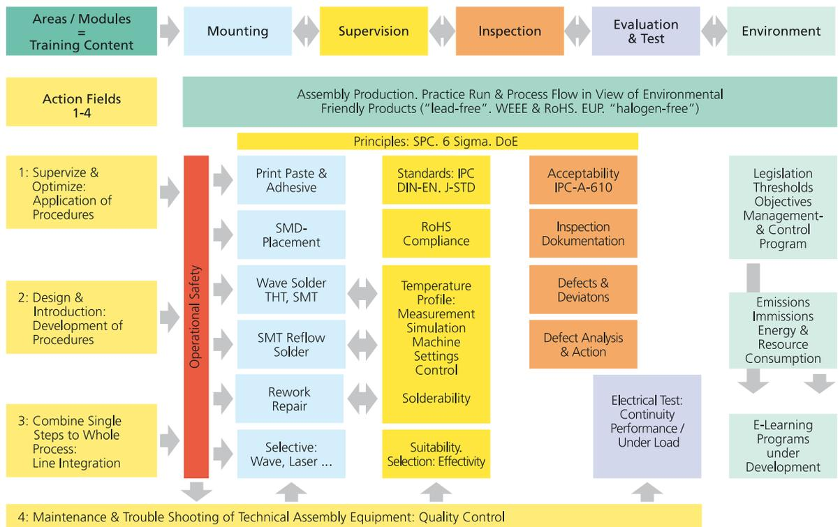
Figure 2: Schematic of the modular training concept.
