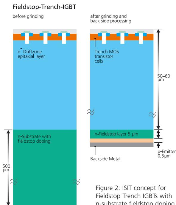
Figure 2: ISIT concept for Fieldstop Trench IGBTs with n-substrate fieldstop doping.
