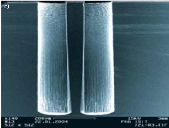
c) The donut structures are etched approx. 550  $\mu\text{m}$  deep into the silicon wafer. Filling the donut structures was more difficult than using pin type wafers.
