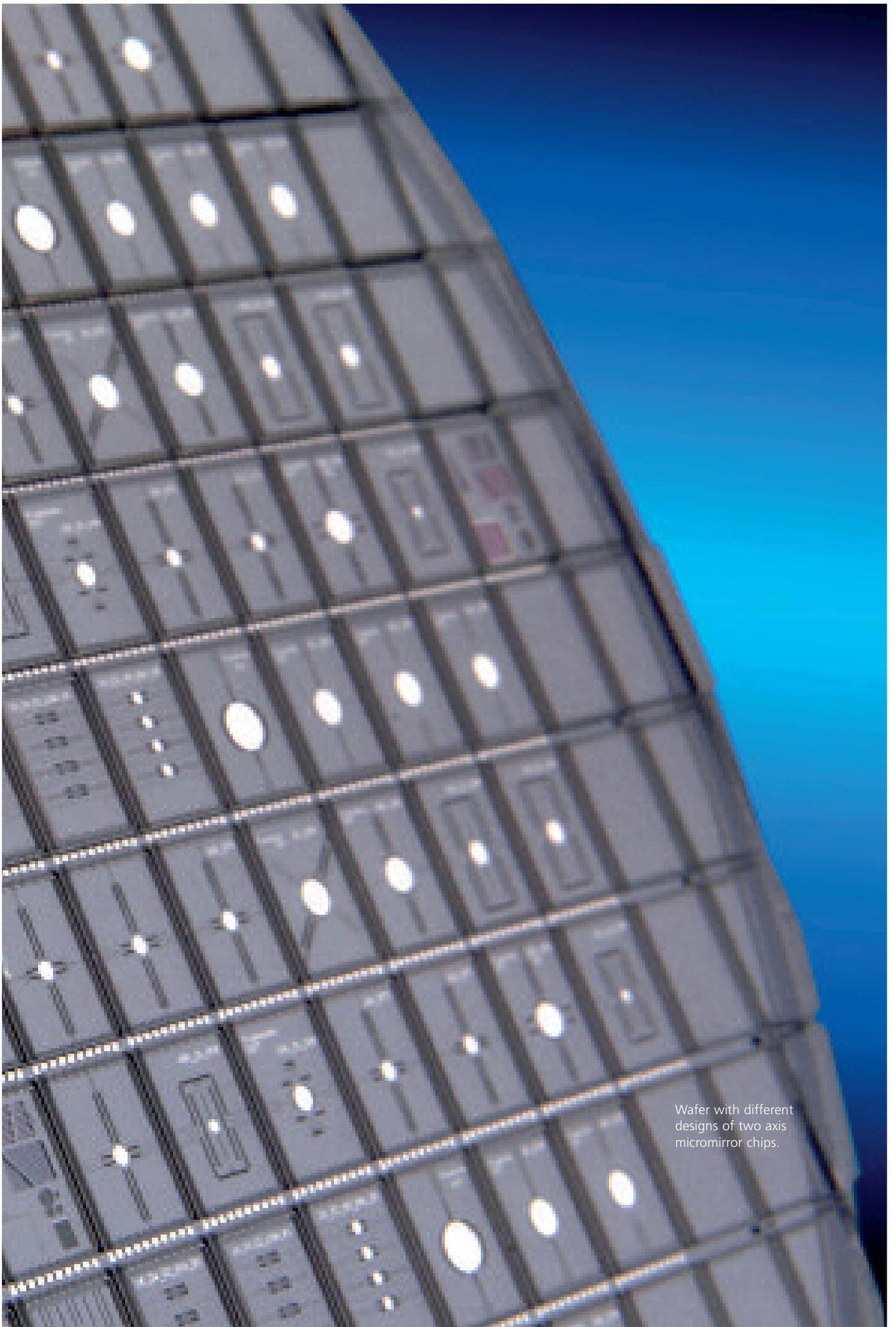
Wafer with different designs of two axis micromirror chips.
