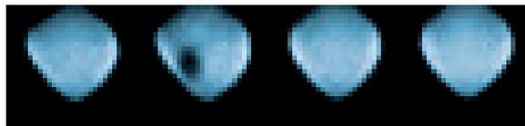
Figure 1: Vertical section through CSP-solder balls from 3D x-ray volume reconstruction.
