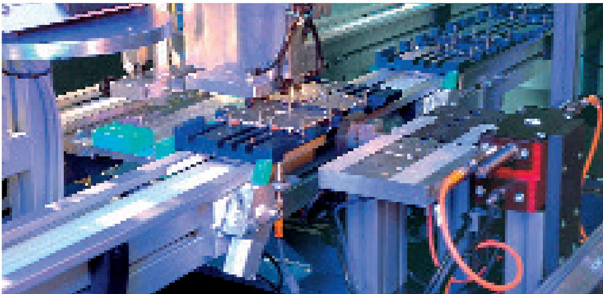
Lithium polymer battery production line: automated stacking of battery layers.
