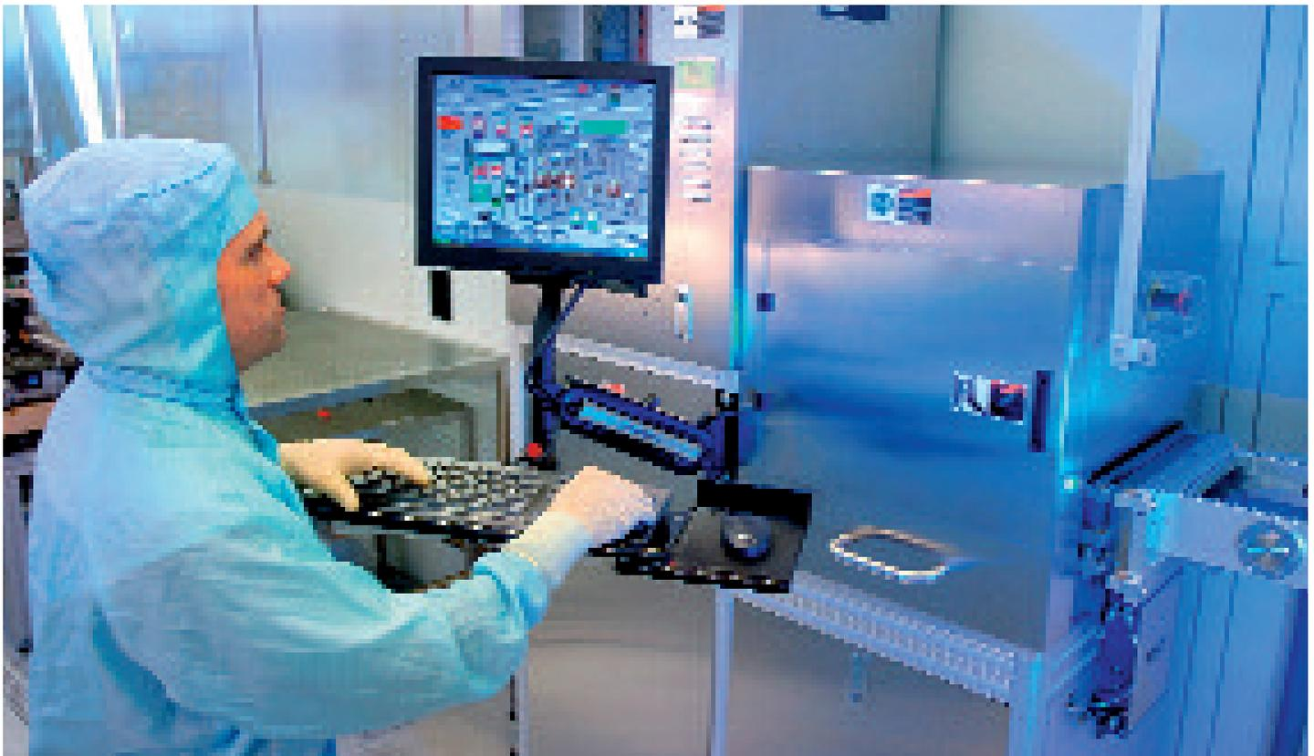
Placing a wafer batch into a spray acid tool for surface cleaning.
