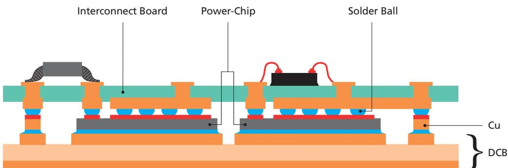
Figure 3: Principle schematic of a sandwich type power module assembly. The power devices are soldered at the front and back side.
