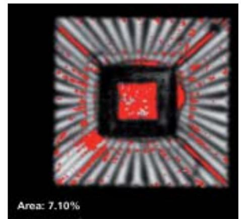
component after the reflow load. Red areas show delamination within the mould compound of package and within the die bond of the chip. If internal cracks are indicated by acoustic microscopy they must be considered a failure or verified good using microsection through the identified site. The corresponding microsection, which is a destructive analysis method, is shown in figure 2. A separation between the leadframe and the die bond is visible.
