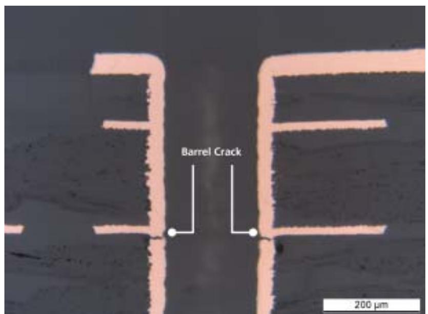
Verification of solder heat resistance of SMD and substrates are performed at the ISIT LEADFREE Training Line. Components and PCB materials can be qualified for customer defined reflow profiles and demands.
