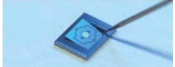
Figure 2: A new mirror design enables permanent static preinclination of the 2D-scanner for spatial separation of reflex and projected image.
