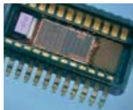
Open cavity package with angular rate sensor and read out ASIC.
