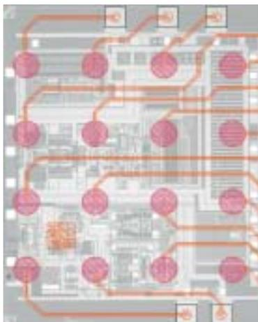
WLP technology can also be applied for packaging sensors under vacuum, such as angular rate or acceleration sensors. ISIT has successfully integrated thin film getter layers for high-Q microresonators and improved vacuum lifetime.
