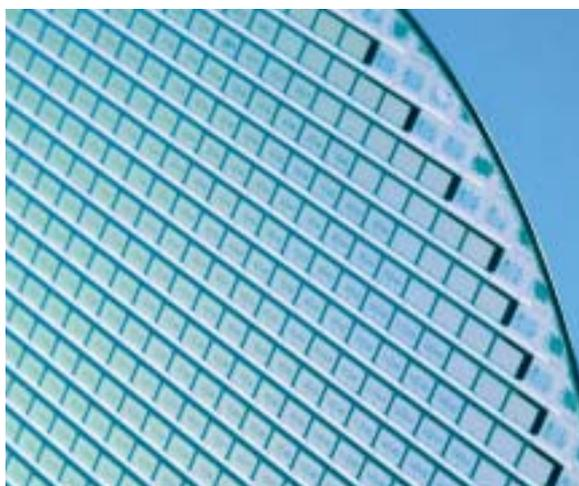
Silicon Wafer with encapsulated micro mechanical gyroscopes.
