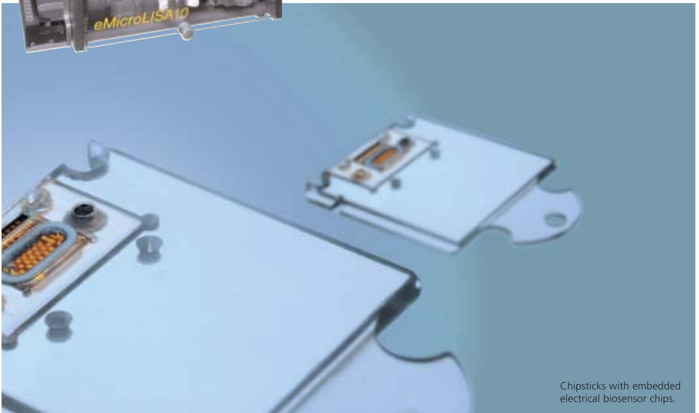
Chipsticks with embedded electrical biosensor chips.
