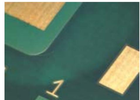
To verify if the substrates withstand this accumulated thermal stress they are exposed 3 – 6 times to a convection reflow process with a maximum substrate temperature of 260° C. An optical inspection is performed to identify delamination or other optical changes of the substrate material. Figure 3 shows a PCB substrate with delaminated areas after 4 times reflow simulation. Electrical tests are performed to verify electrical parameters, like value of resistance.
