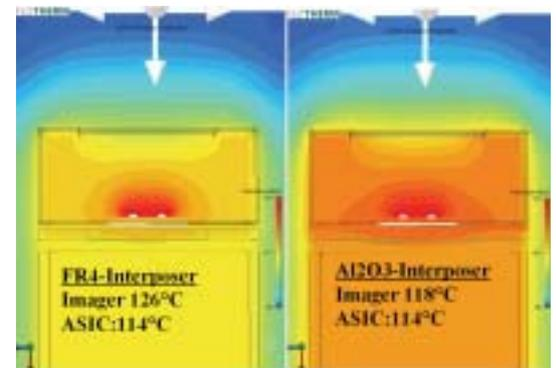
Figure 3: With 95°C ambient air temperature and max. 120°C for the imager, cooling becomes critical. Imager and ASIC are mounted on a ceramic heat-spreader. The thermal simulation shows that a good lateral distribution can be achieved if a good thermal contact between chip and substrate is given.
