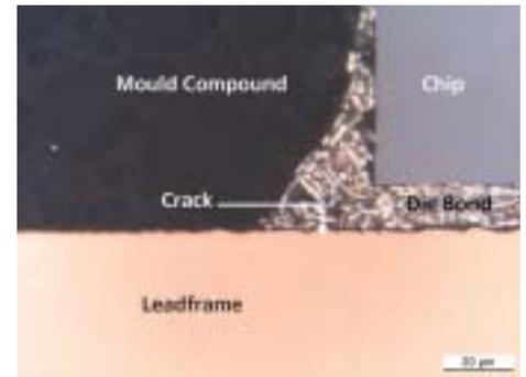
Due to several high temperature soldering processes PCB substrates are exposed to several thermal loads. The typical electronic assembly has to pass through during its production at least two reflow cycles and one selective soldering process. If there is a defective component like a BGA or QFN on the assembly two more reflow cycles are necessary to change this component.
