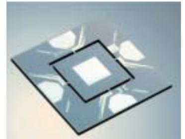
Force/torque sensors: Sensor in test setup (top); part of a wafer with sensors (left); single sensor (right).
