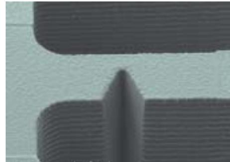
silicon structures the material attrition effects nanoscaled particles as seen with high resolution scanning electron microscopy in figure 2. The development of protective thin film hard coatings for high wear resistance can hereby be monitored directly.
