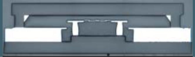
Figure 3: Cross section of a waferlevel packaged 2D microscanner.
