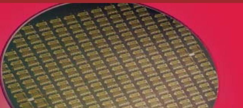
*Silicon wafer with electrical biochips*
