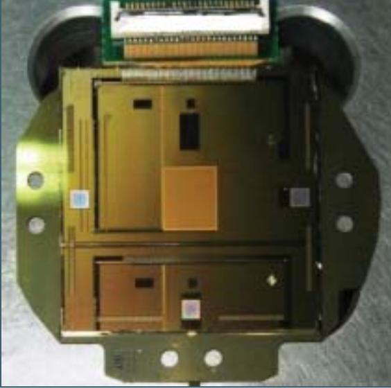
Figure 7: Assembled aperture plate system.
