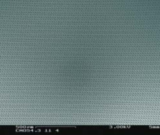
Figure 5: Top view of electroplated blanking and shielding electrodes close to apertures.
