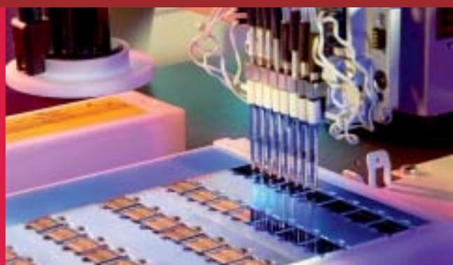
*Spotting process of different liquids on biochips*
