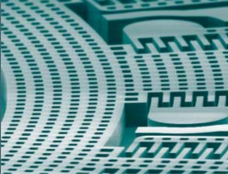
Figure 4: Surface micro machined sensor structure in 11 µm thick polysilicon. The finger electrodes shown in the right are for driving the sensor ring structure. The minimum linewidth of the electrodes is 2 µm.
