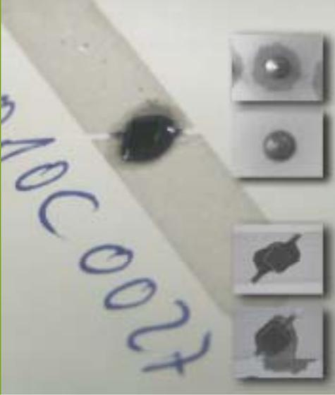
Figure 4: Paper can even be used to fabricate low cost chip modules. The insets show how material selection (underfill, silver epoxy) affects the result.
