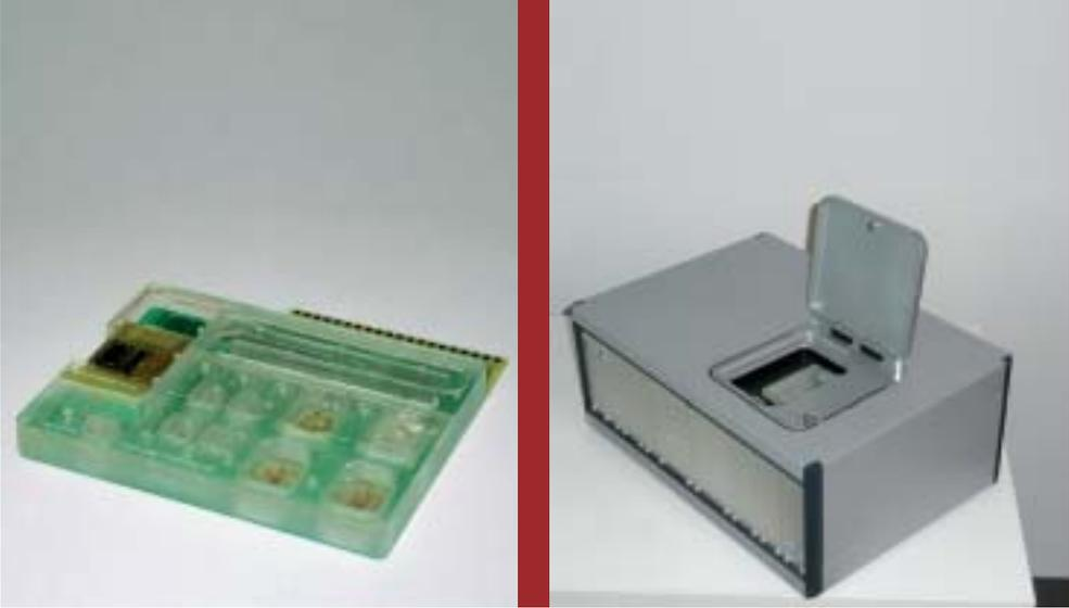
Figure 2a: ivD-cartridge equipped with reservoirs, fluidic parts and chip. Figure 2b: ivD-Measurement device.
