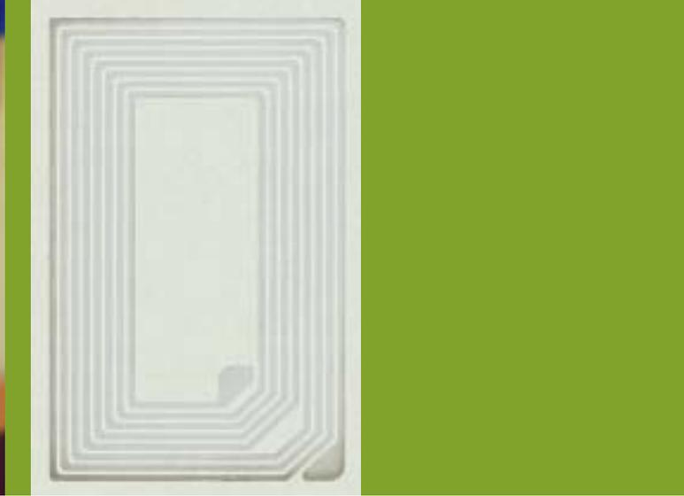
Figure 3: A 13,56 MHz antenna coil, screen printed on paper as a substrate. The pads connect it to a chip module (figure 4).
