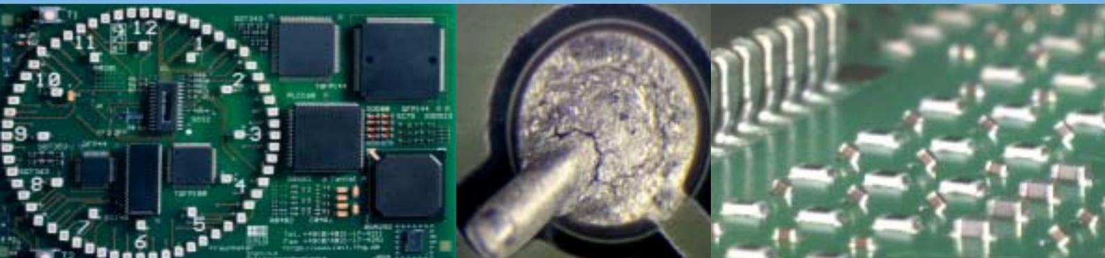
*ISIT test board for soldering process evaluation*
