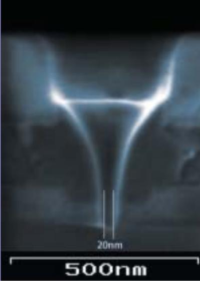
Realization of nano holes in the sub 20 nm regime by side wall spacer formation using amorphous Si.
