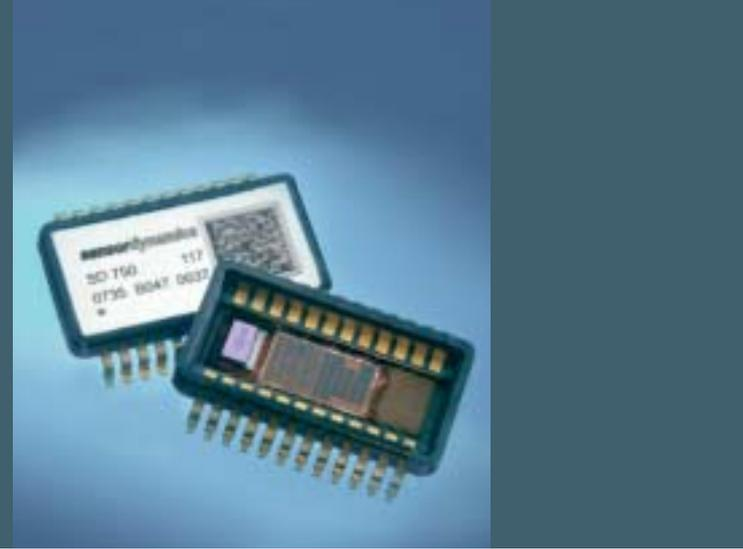
Figure 2: The open cavity OC24 housing includes a combined MEMS Sensor chip (left) and an ASIC (right). The single chip MEMS sensor integrates one accelerometer and one angular rate sensor.
