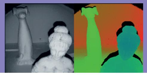
Figure 3: Different working modes of the camera. Left: Reflected light intensity, Right: Phase shift between light source and reflection
