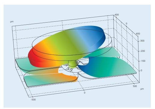
Figure 3: The patented "rose-leaf" actuator with suspension structures minimizes the pitch size and improves mechanical linearity
