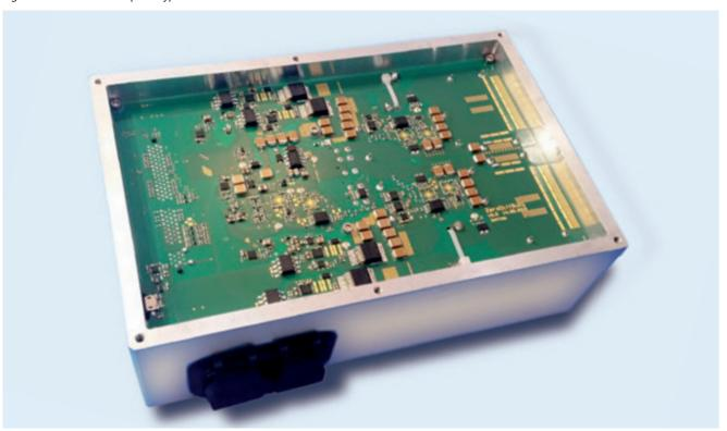
Figure 1: 2.5 kW inverter prototype
