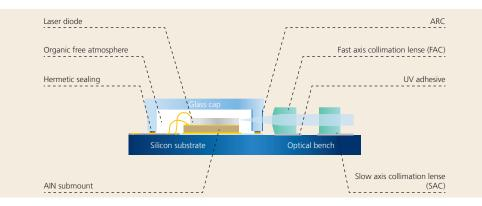
Figure 1: Schematic cross section of a miniaturized WLP laser module with an optical bench
