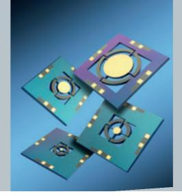
Different types of piezoelectric micromirrors
