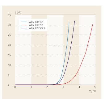
Figure 6: Threshold voltage ( $V_{tr}$ ) of semi-vertical GaN devices of different size and different geometry
