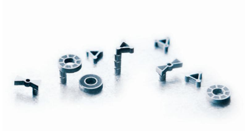
NdFeB micromagnets embedded in silicon
