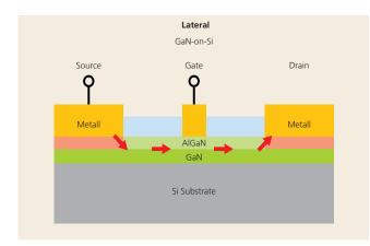
Figure 1a: Schematic of a lateral GaN HEMT device; red arrows show the current path
