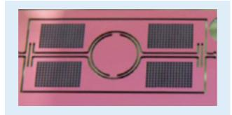
Figure 4: Quasi-static MEMS mirror actuator using four arrays of embedded permanent micro-magnets
