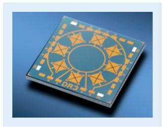
Figure 3: MEMS chip for ultrasonic application
