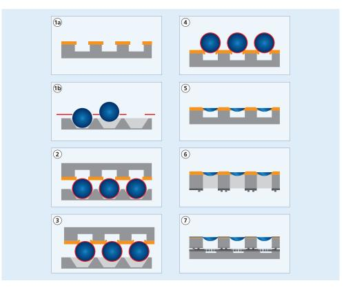
Figure 2: Process flow to integrate Si lenses on the wafer level
