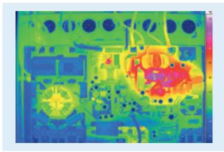
Figure 2: Heat image of a defect coil
