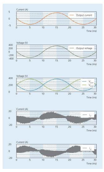
Figure 2: Measured output voltage and frequency modulated inductor currents
