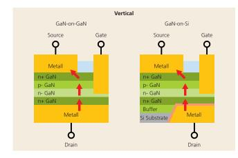
Figure 1b: Schematic of vertical GaN devices; red arrows show the current path
