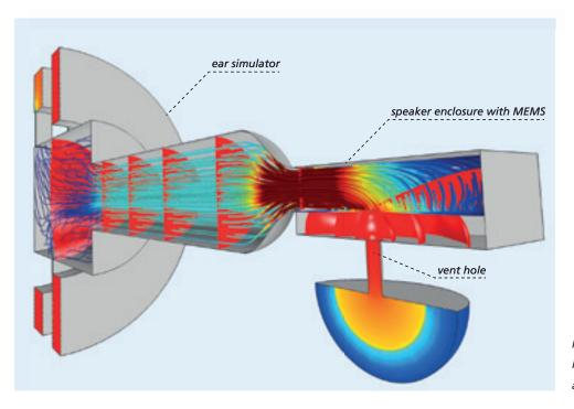
Figure 4: FEM simulation of a MEMS in-ear speaker coupled to an ear simulator
