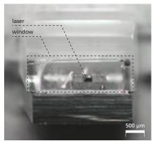
Figure 4: Front view through the emission window on a packaged laser diode
