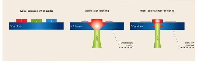
Figure 6: Concept of in-situ laser soldering with direct heat transfer to the soldering pad of a laser diode to further reduce the placement pitch by reduced heat spreading
