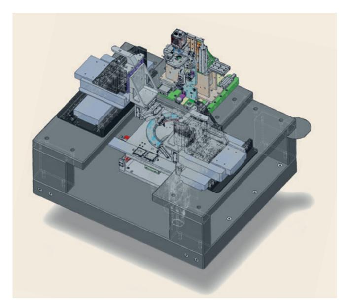
Figure 5: CAD construction overview on functional modules in the design process of a new ultraprecision assembly station with integrated in-situ laser soldering and active alignment functionality
