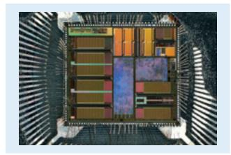
Figure 3: Wet-etch opened chip package
