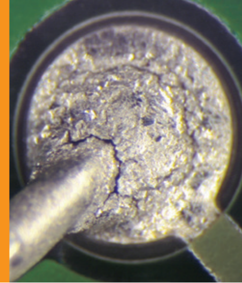
THT-solder joint with fatigue crack
