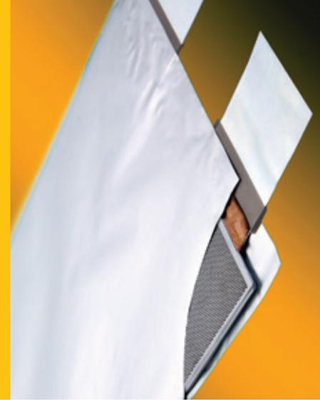
*Contacting- and feed-through area of a pouch cell*
