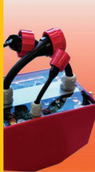
*1 kWh battery module in autonomous operating vehicles for deep sea exploration*
